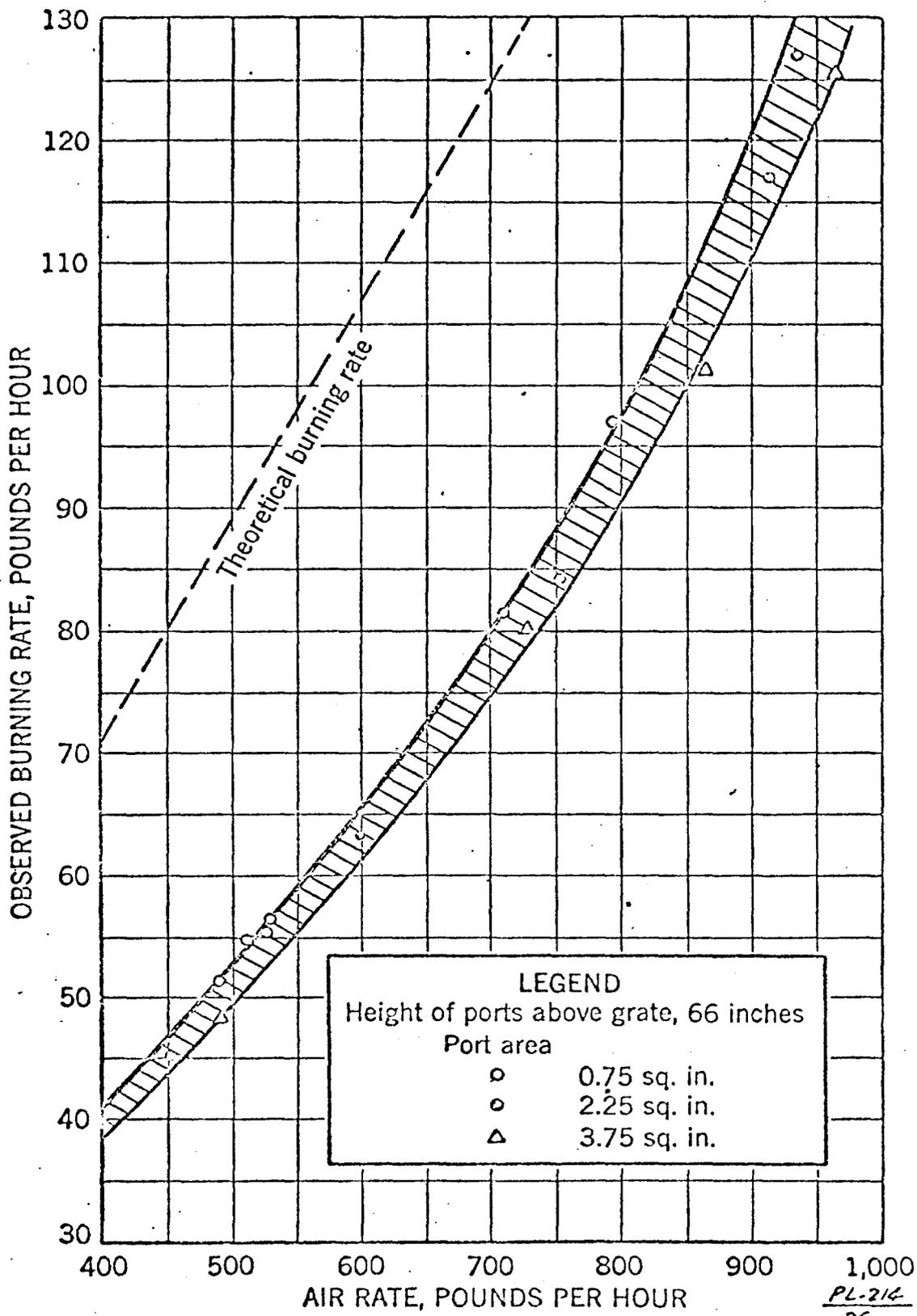
Figure 11. Average observed burning rate as a function of air rate.
