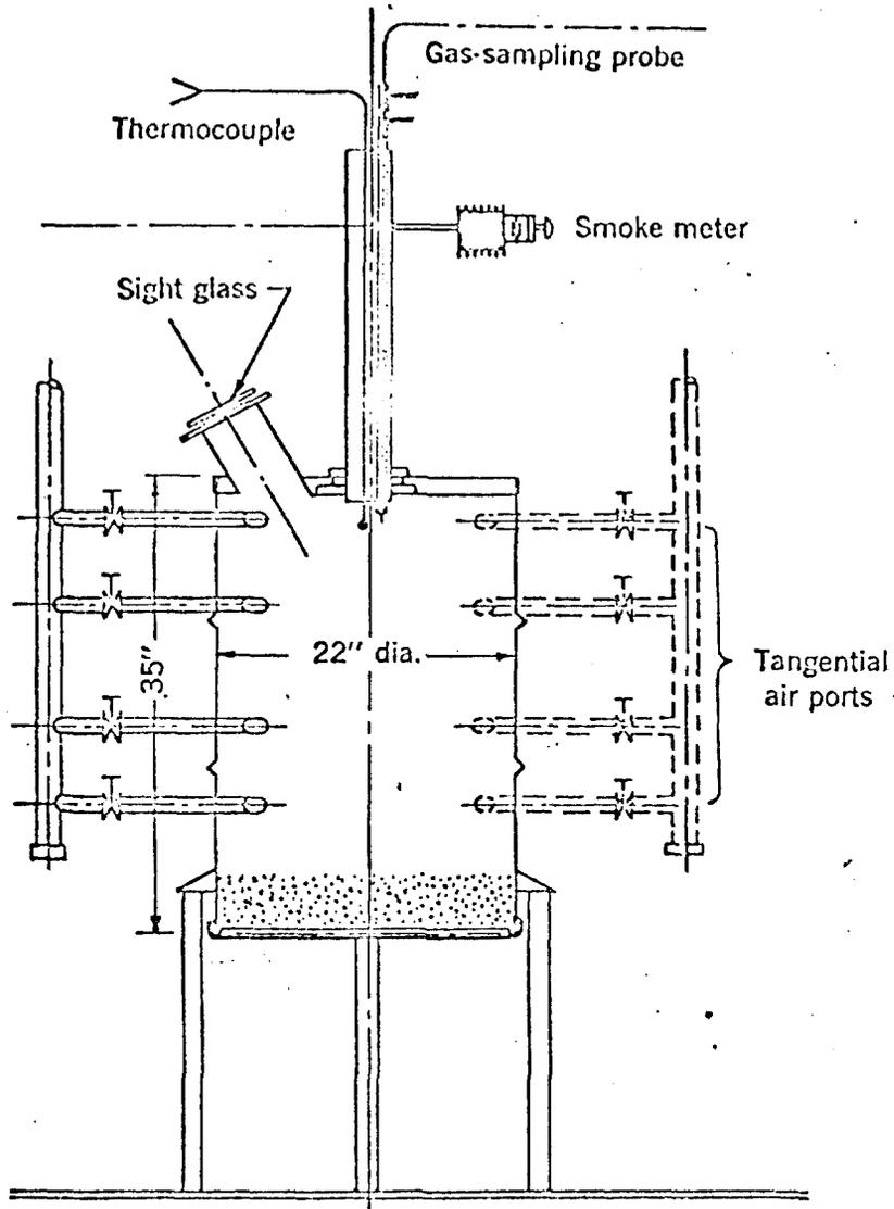
Figure 1. Schematic diagram of model incinerator.
