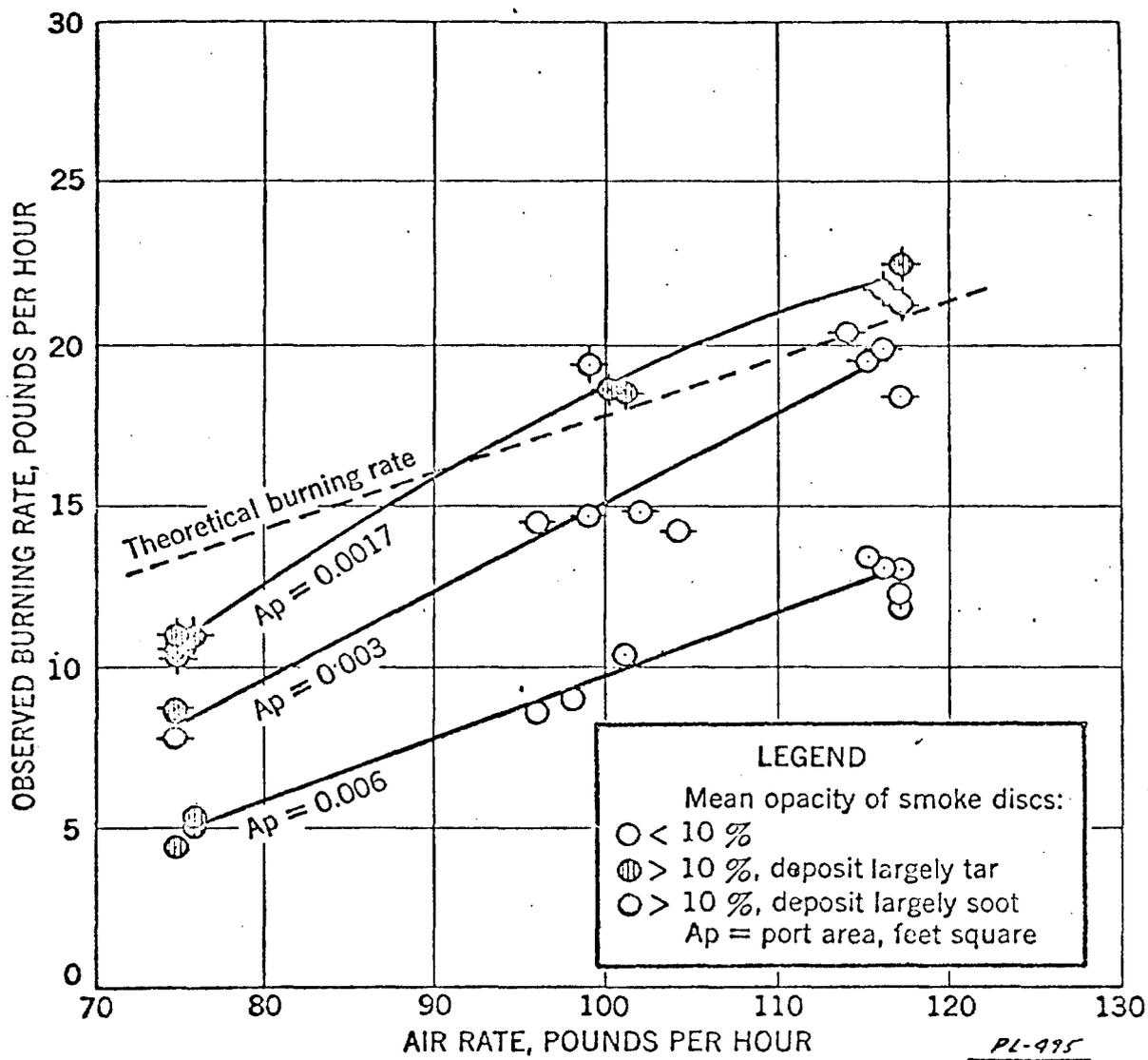
Figure 2. Average observed burning rate as a function of air rate and port area.
