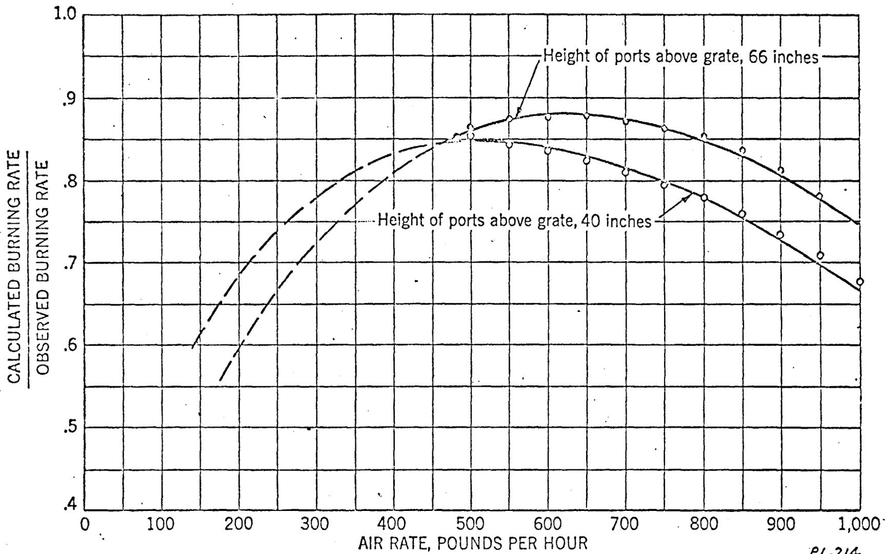
Figure 13. Combustion efficiency as a function of air rate.
