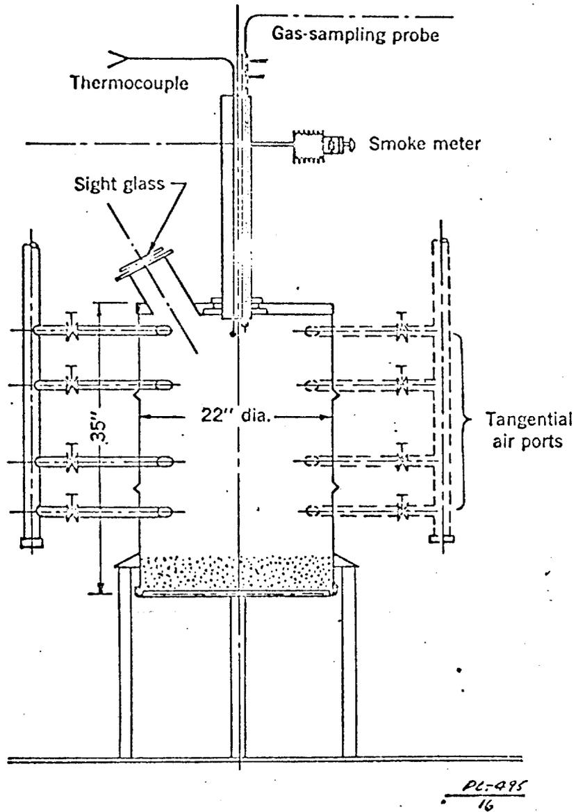
Figure 1. Schematic diagram of model incinerator.
