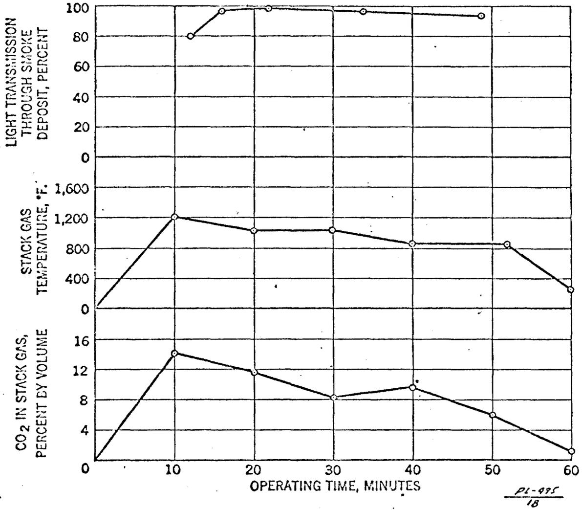
Figure 7. Operating conditions for a Reynolds number of 19,400, air rate = 117 pounds per hour.
