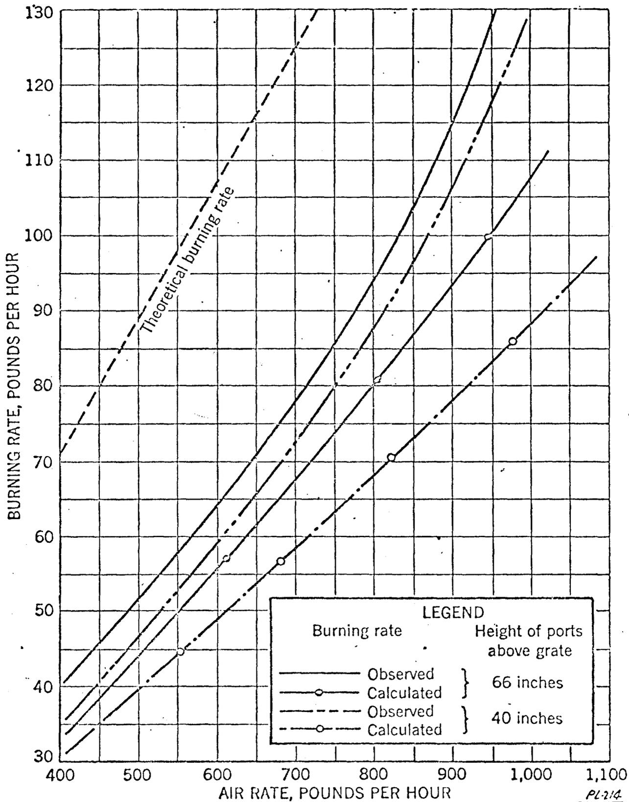
Figure 12. Burning rate as a function of air rate and port height.
