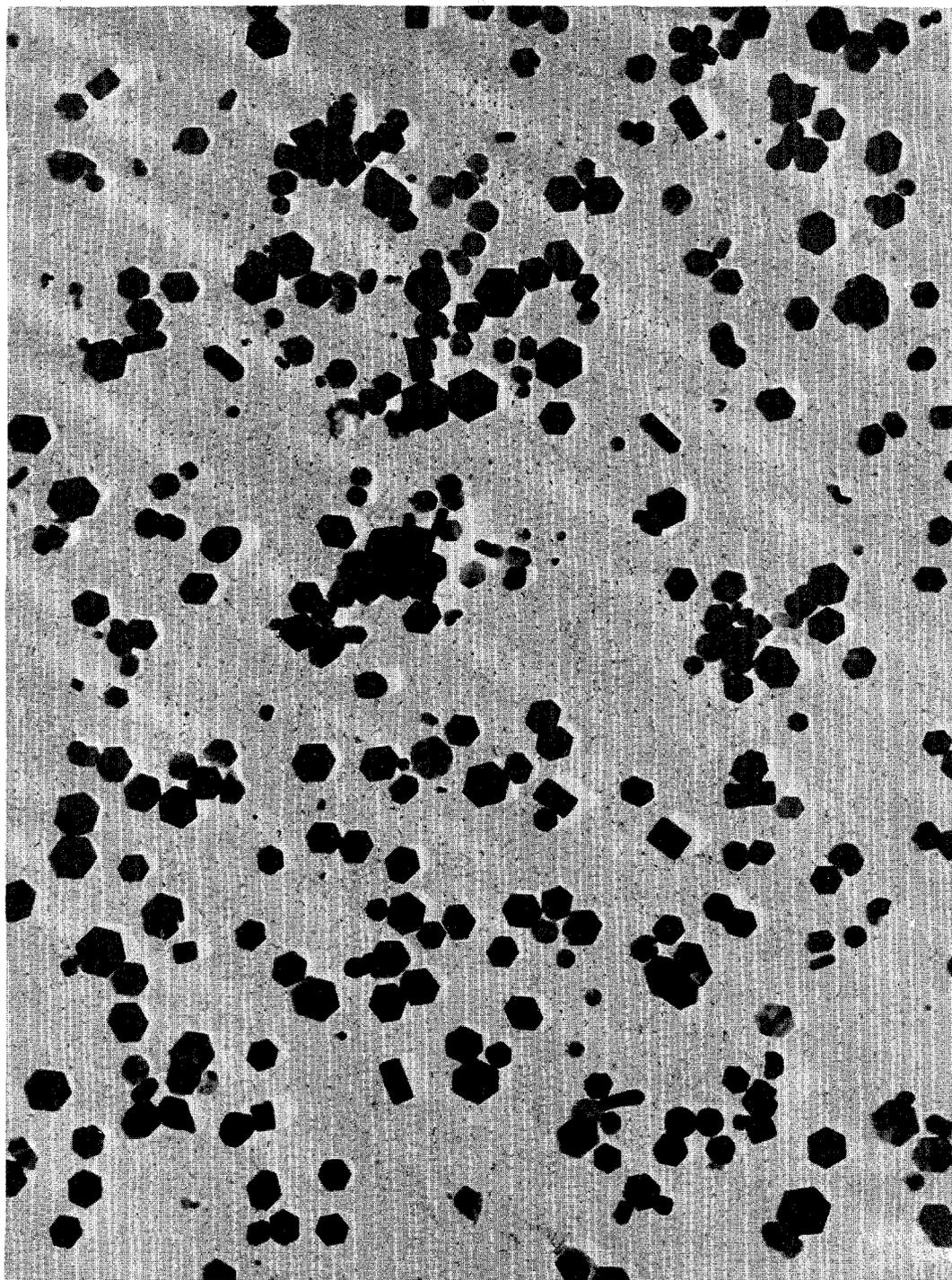
Replica of crystalline  $U_3O_8$  particles vaporized from  $UO_2$  melted in air. 40,000X. (Particle diameters 0.02 to 0.2 microns.)
