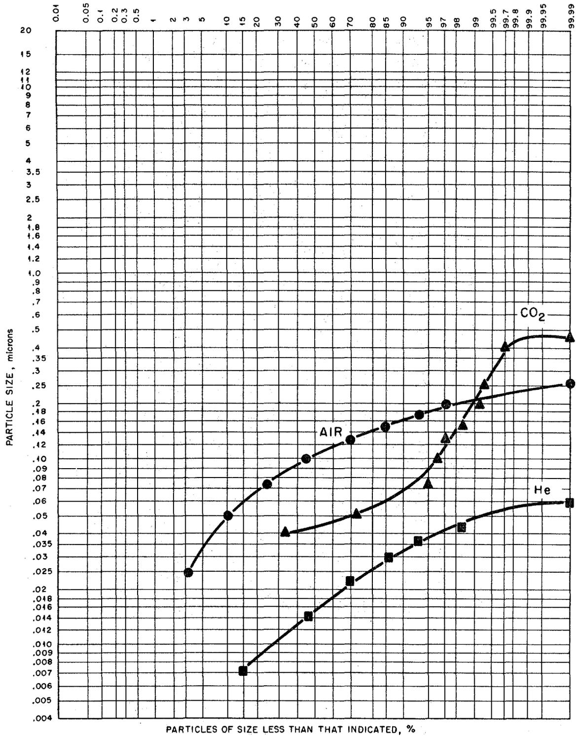
Particle Size Evolution of Oxides Vaporized from Melted UO<sub>2</sub>. (Arc-image Furnace).
