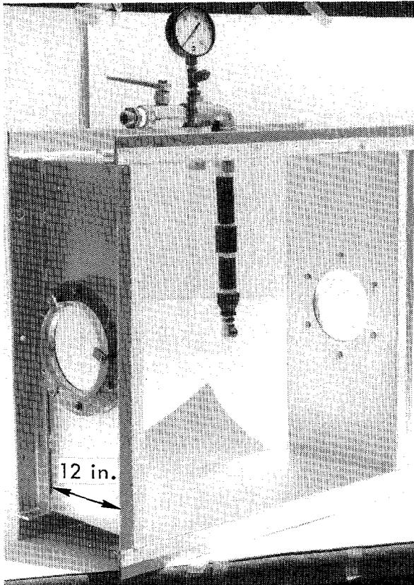
Fig. 11. Twelve-in. duct section, showing one spray system.
