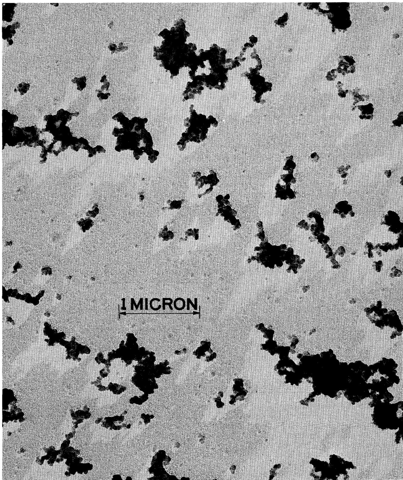
Figure 12. Smoke particles from 70 percent normal paraffin hydrocarbon, 30 percent tributyl phosphate fire
