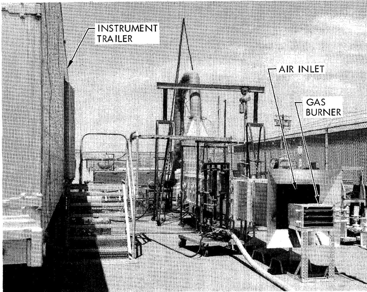
Fig. 3. View of spray damper experimental setup from fire end.
