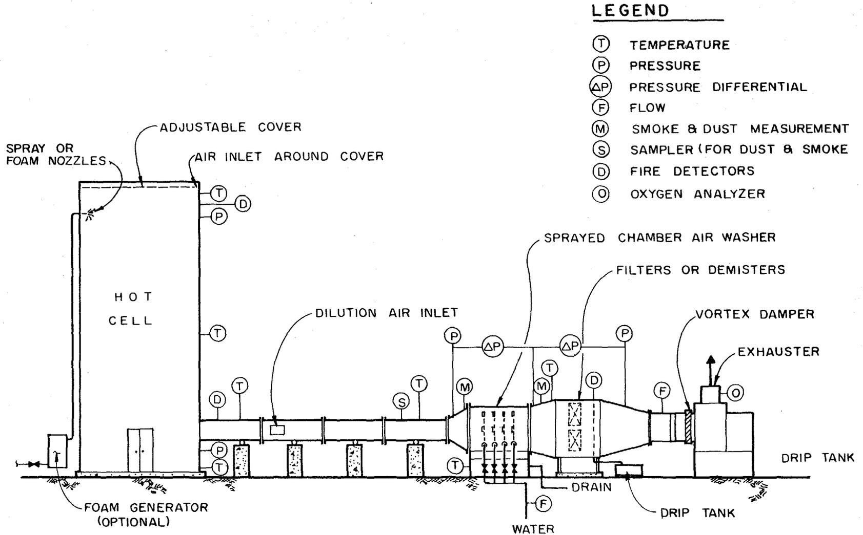
**DIAGRAM OF FIRE TEST FACILITY**
