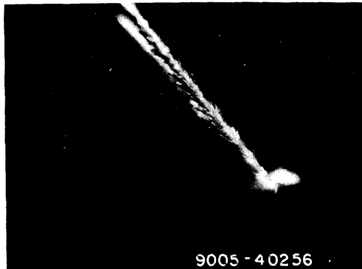
Figure 11. Dendritic column of sodium oxide formed on impact plate.
