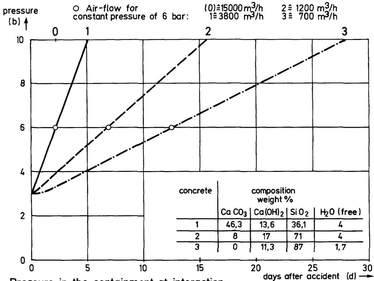
Pressure in the containment at interaction of concrete and melt as a function of time (calculated by M.Reimann IRB/KfK with „Wechsel“)
