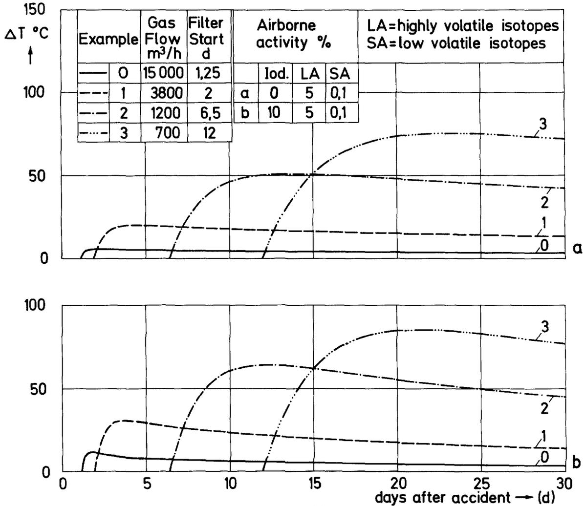
Temperature rise of exhaust air filter system after an accident as a function of time
