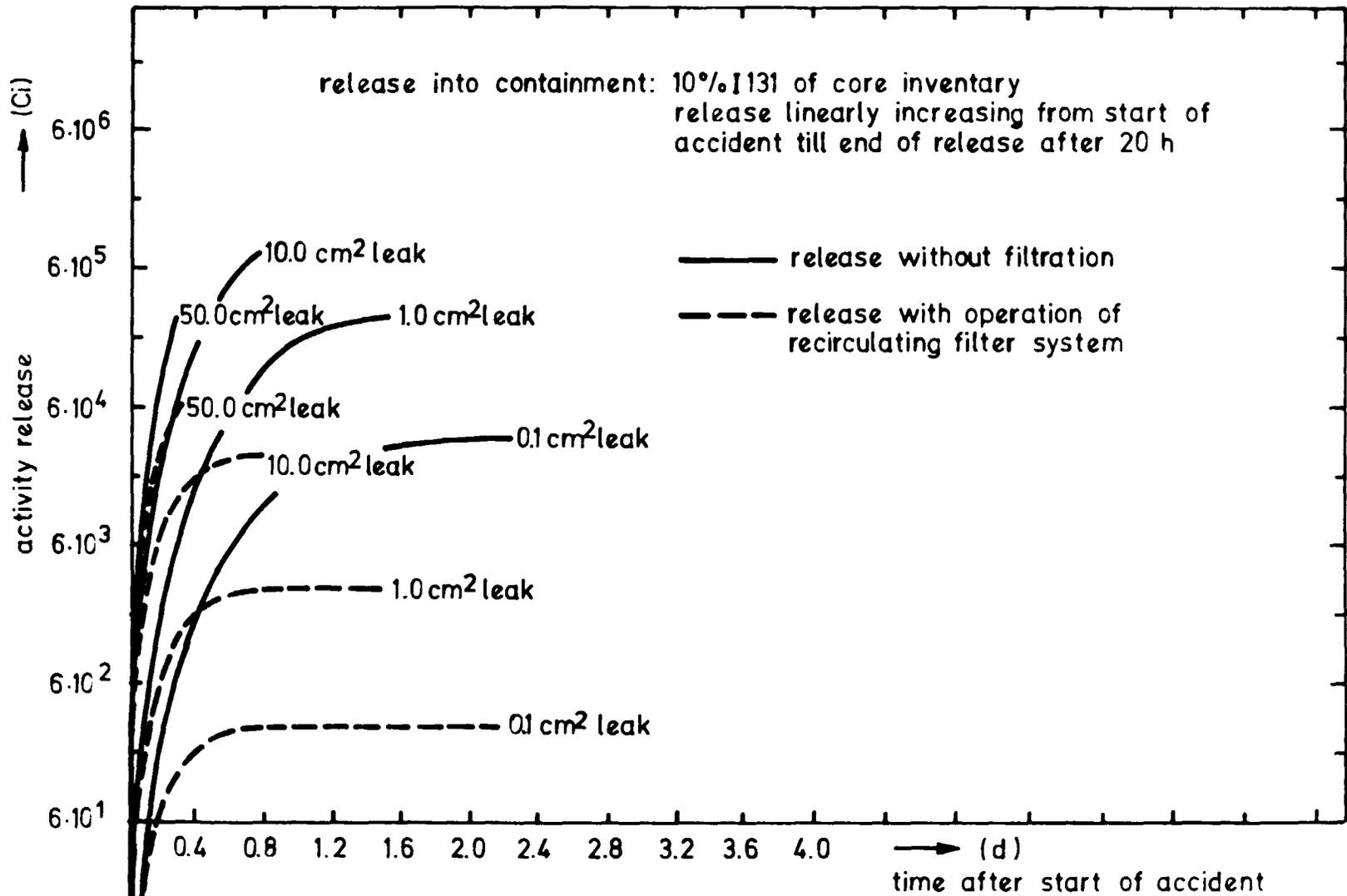
activity release into annular compartment at different leak areas - filter volume flow = 20 000 m<sup>3</sup>/h
