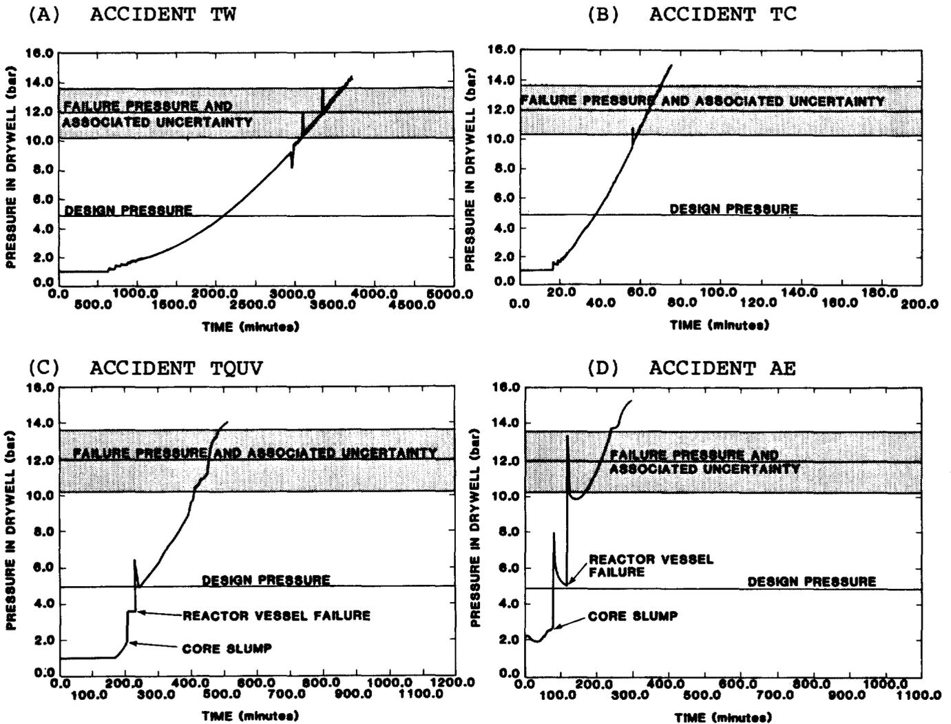
Figure 3 MARCH Code Calculations of Containment Pressure Versus Time for Four Hypothesized Accidents in the Baseline BWR Plant
