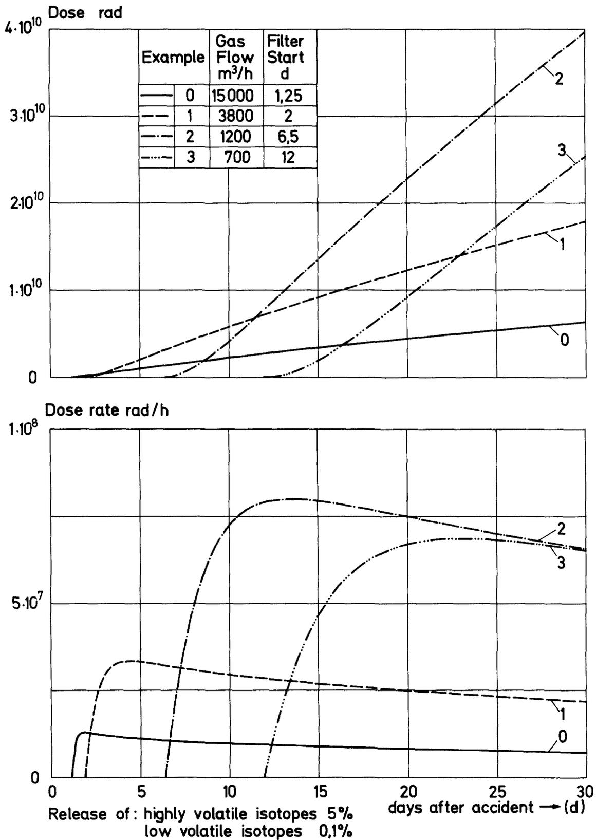
Dose and Dose rate of the HEPA filter after an accident as a function of time
