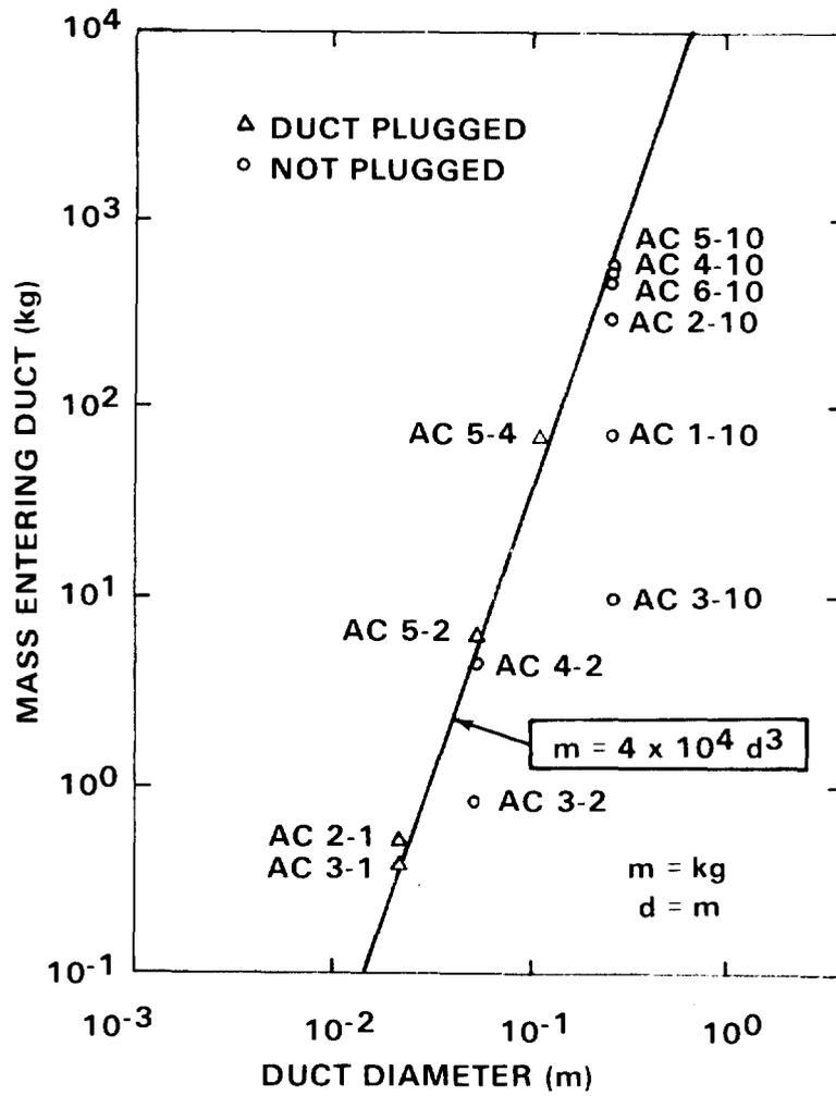
FIGURE 6. Duct Plugging as a Function of Duct Diameter.
