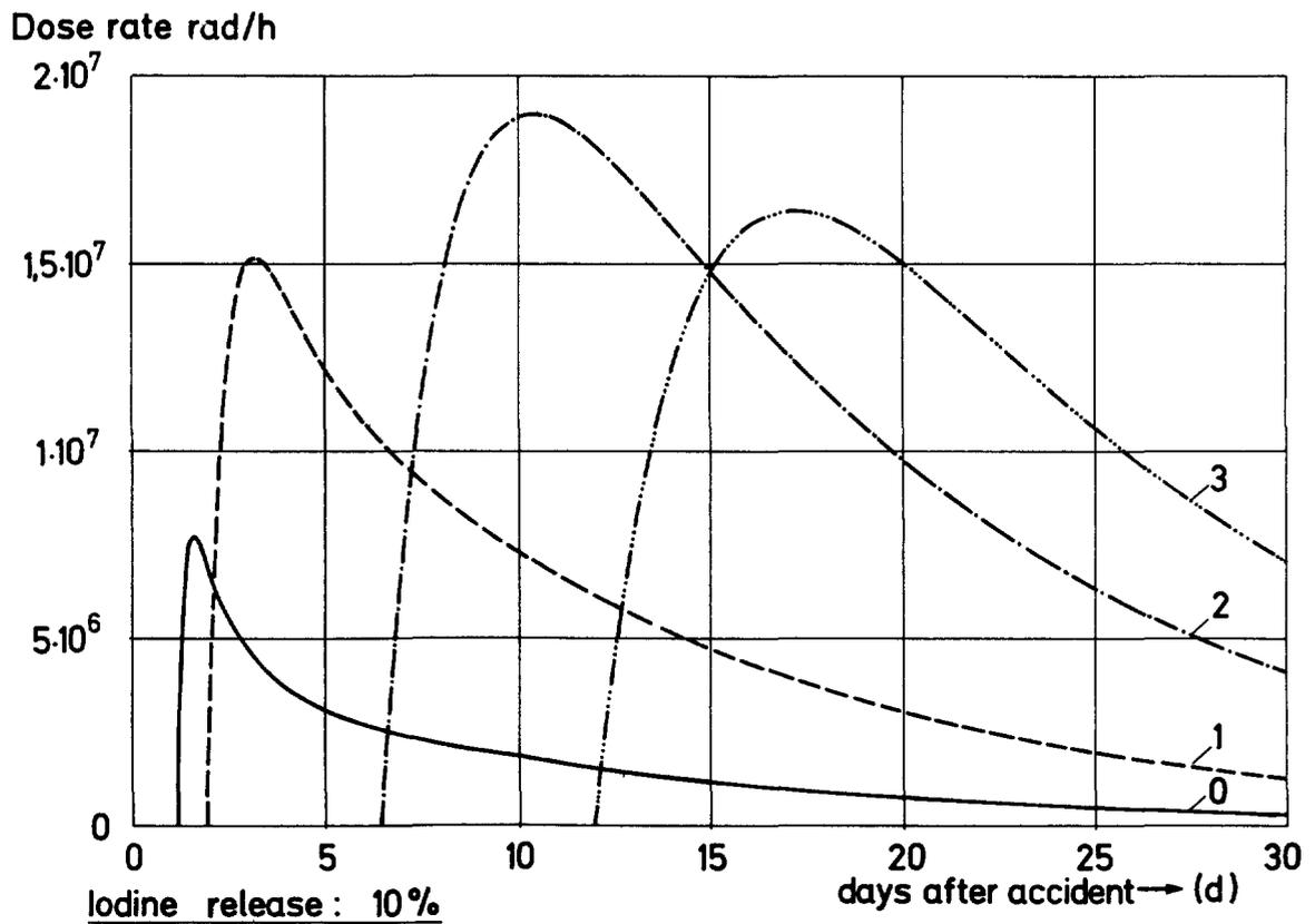
Dose and Dose rate of the iodine filter after an accident as a function of time
