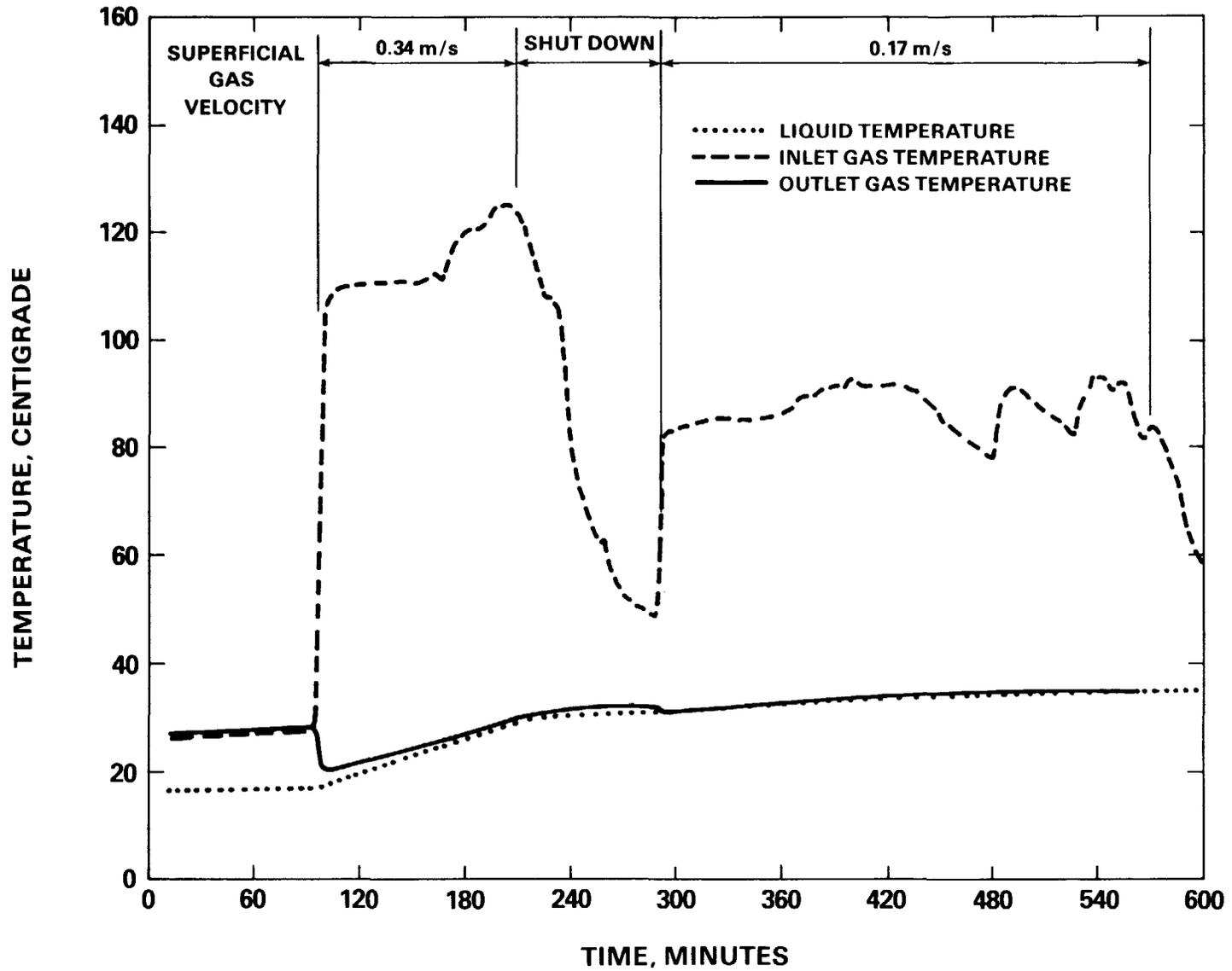
Figure 6. Gas Cooling by the SGS.
