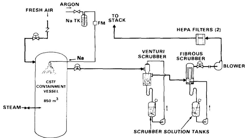
FIGURE 3. Flow Diagram of the CSTF Scrubber Air Cleaning System Used in Tests AC-5 and AC-6. (Neg. 8010843-3)
