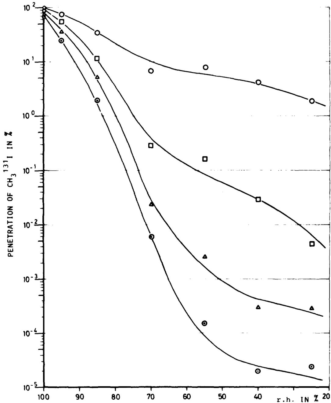
PENETRATION OF AC 6120 BY CH<sub>3</sub><sup>131</sup>I AS A FUNCTION OF THE RELATIVE HUMIDITY OF THE AIR (7)
