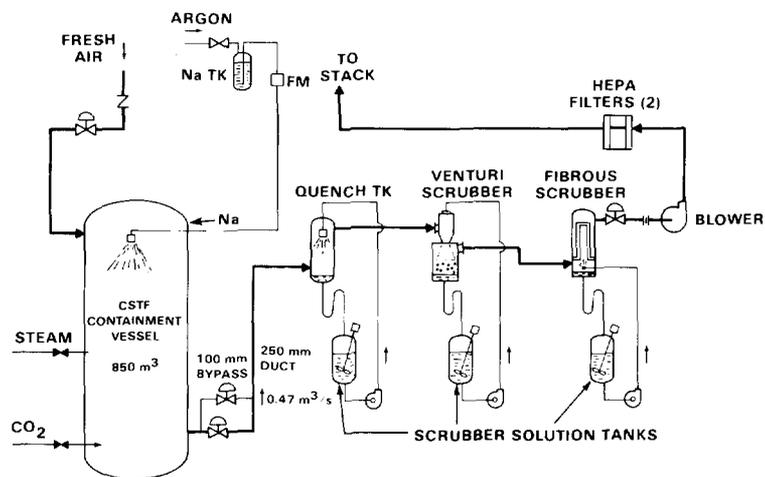
FIGURE 1. Flow Diagram of the CSTF Scrubber Air Cleaning System Used in Tests AC1-AC4. (Neg. 8010843 - 2)
