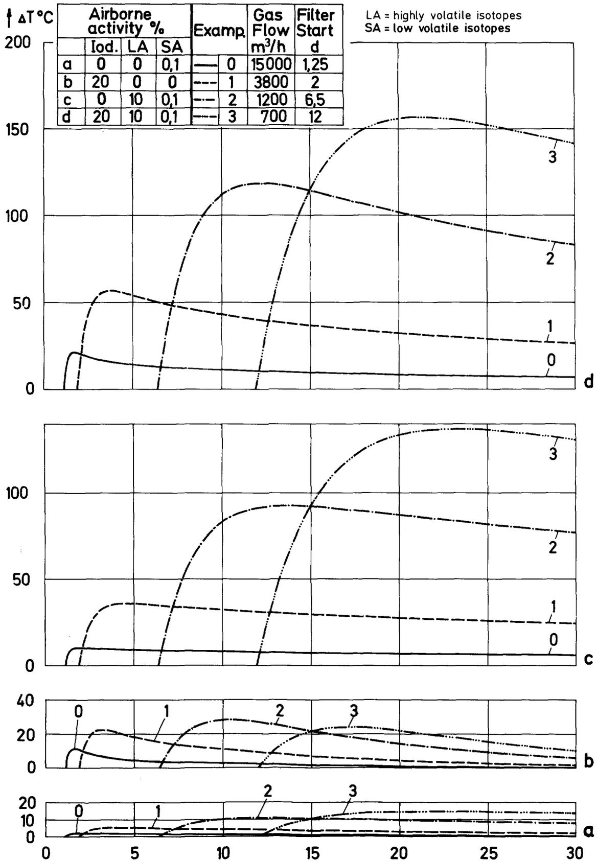
Temperature rise of exhaust air filter system after an accident as a function of time
