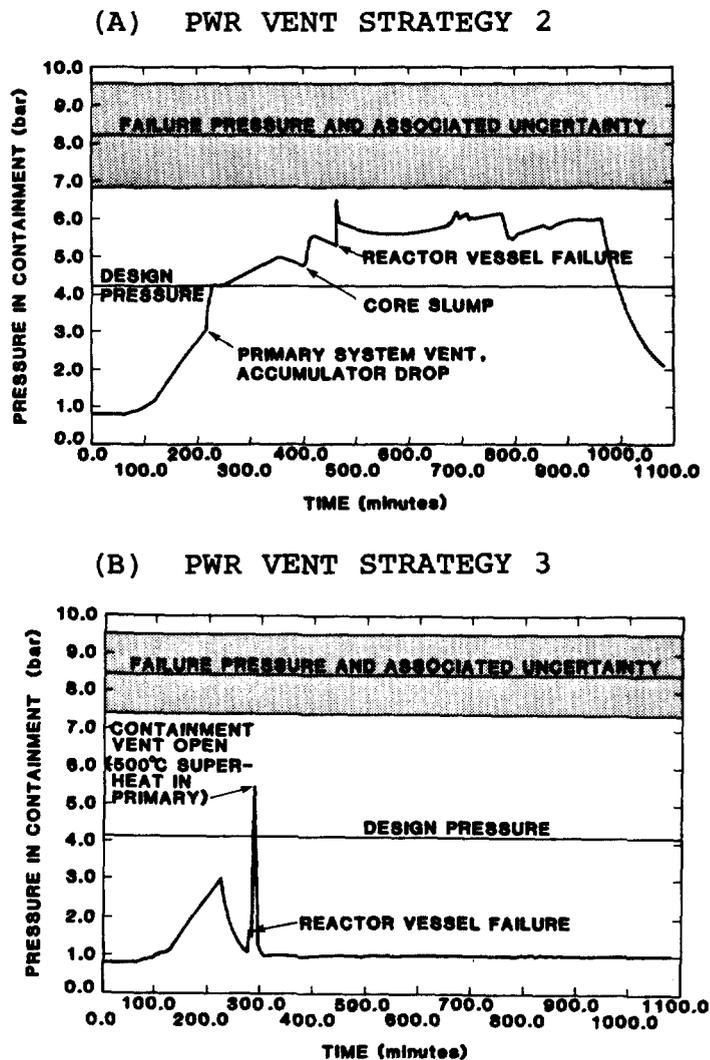
Figure 2 MARCH Code Calculations of Containment Pressure Versus Time for the Accident 'TMLB' in the Baseline PWR with Different Venting Strategies
