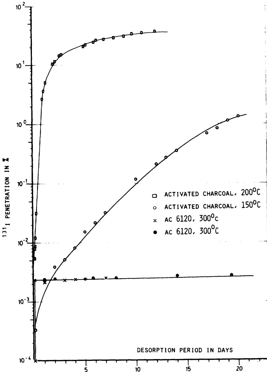
$^{131}\text{I}$  DESORPTION OF VARIOUS ADSORBERS AT ELEVATED TEMPERATURES 7)
