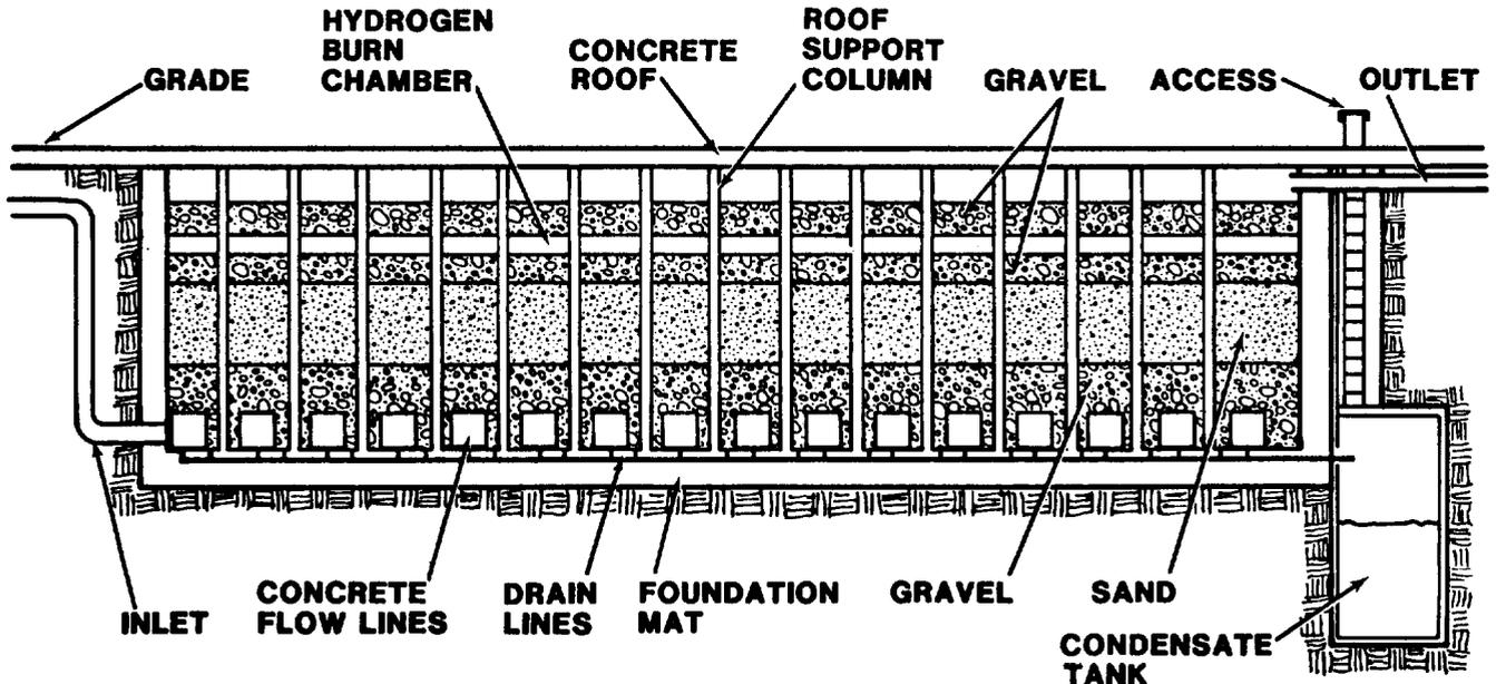
Figure 8 Sand-Gravel Filter Section
