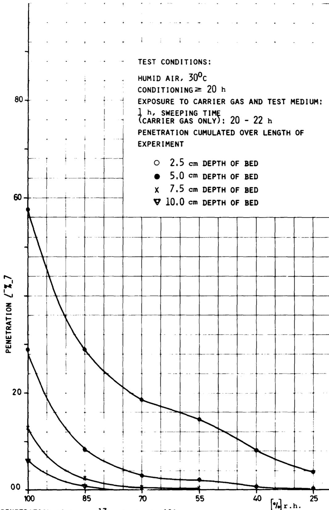
PENETRATION OF LINDE 13 x Ag BY CH<sub>3</sub><sup>131</sup>I AS A FUNCTION OF THE RELATIVE HUMIDITY OF THE AIR 7)
