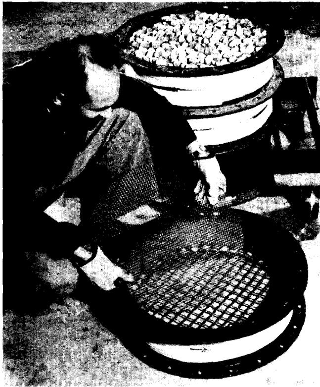
FIGURE 3. Filter Stack Aggregate Trays.
