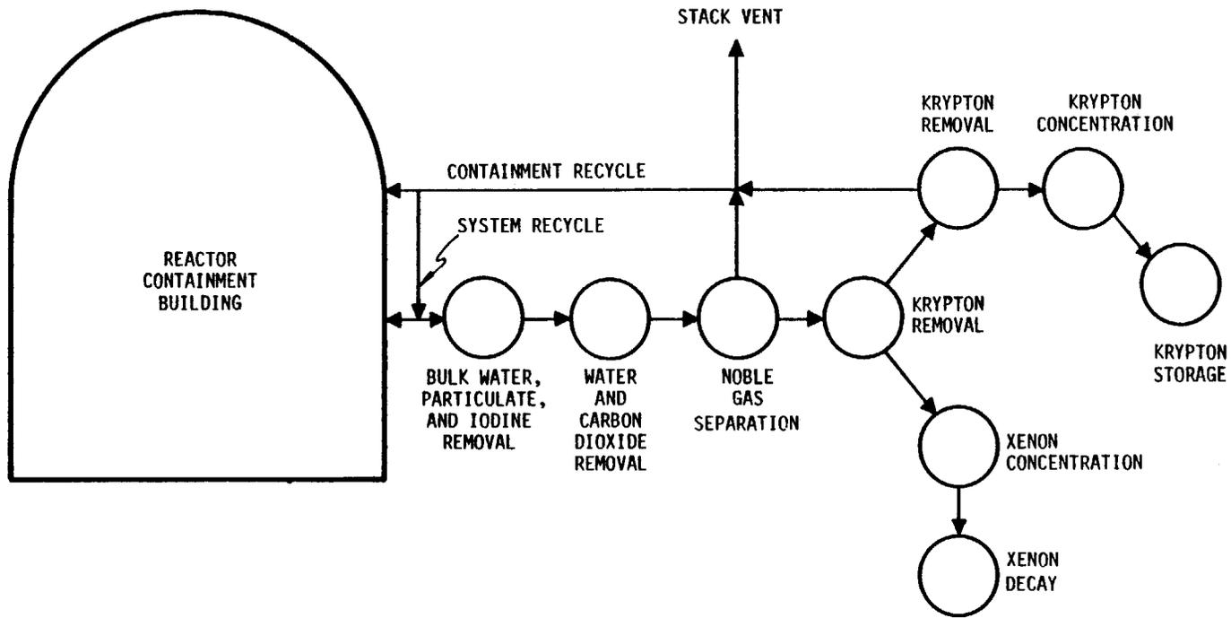
Figure 2. Emergency Noble Gas Recovery System Using Selective Adsorption
