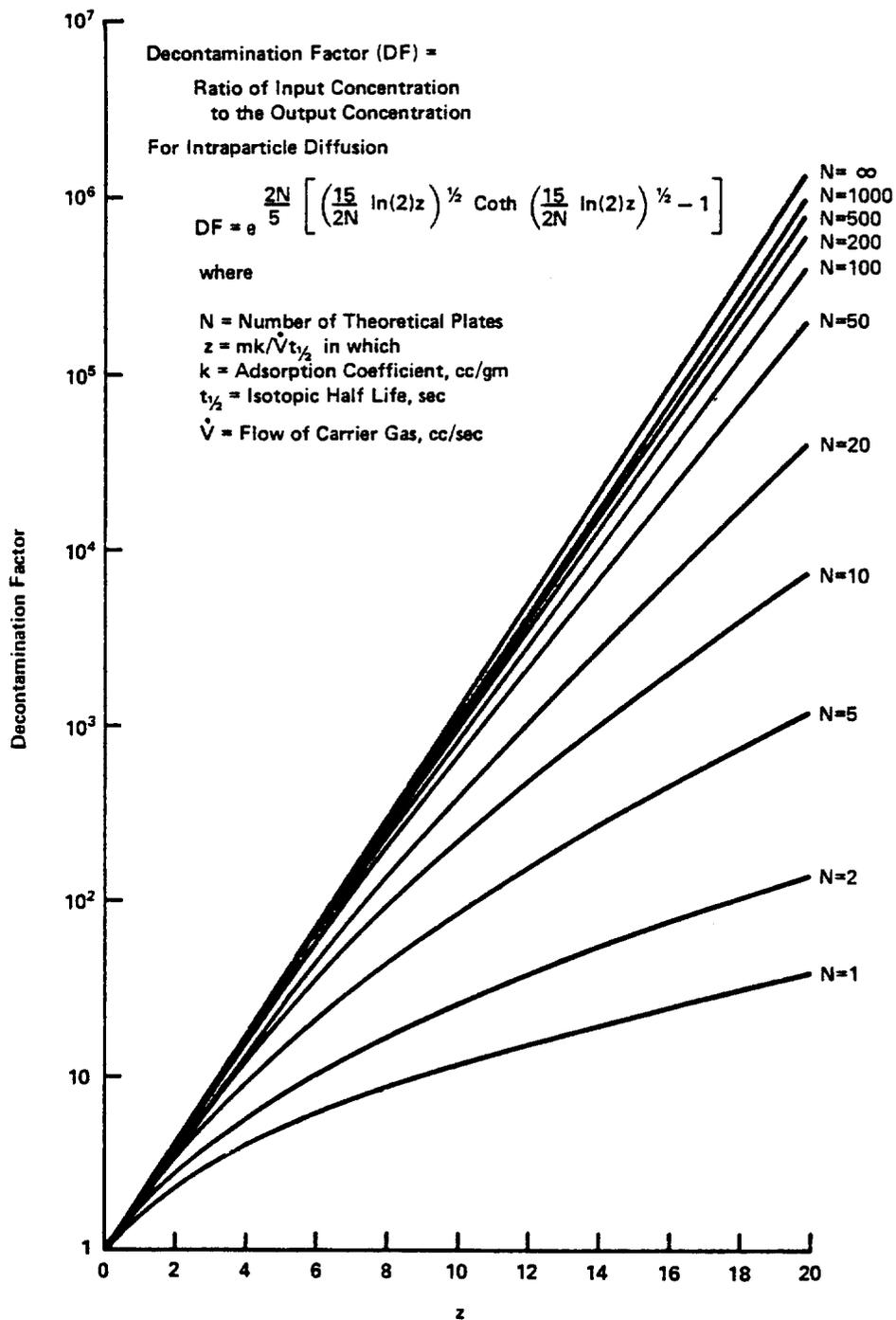
Figure 7 Effect of Intraparticle Diffusion on the Decontamination Factor
