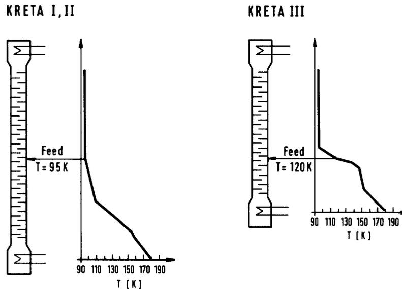
**FIGURE 1 Feed Points and Temperature Profiles in KRETA Columns**
