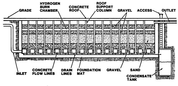
Figure 8 Sand-Gravel Filter Section
