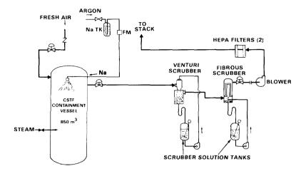
FIGURE 3. Flow Diagram of the CSTF Scrubber Air Cleaning System Used in Tests AC-5 and AC-6. (Neg. 8010843-3)
