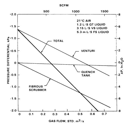
FIGURE 5. Differential Pressure Across Three-Component Scrubber System. (Neg. 8010843-1)
