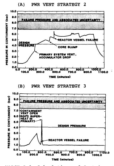
Figure 2 MARCH Code Calculations of Containment Pressure Versus Time for the Accident TMLB' in the Baseline PWR with Different Venting Strategies
