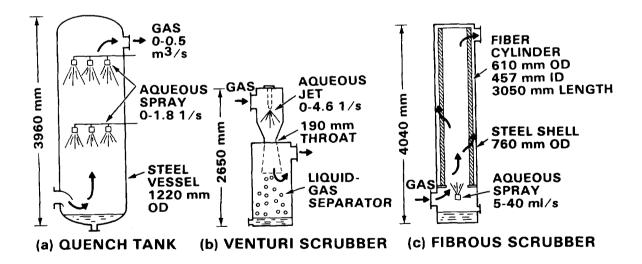
FIGURE 4. Details of CSTF Aqueous Scrubber Components. (Neg. 8010845-1)
