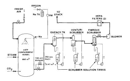
FIGURE 1. Flow Diagram of the CSTF Scrubber Air Cleaning System Used in Tests AC1-AC4. (Neg. 8010843 - 2)
