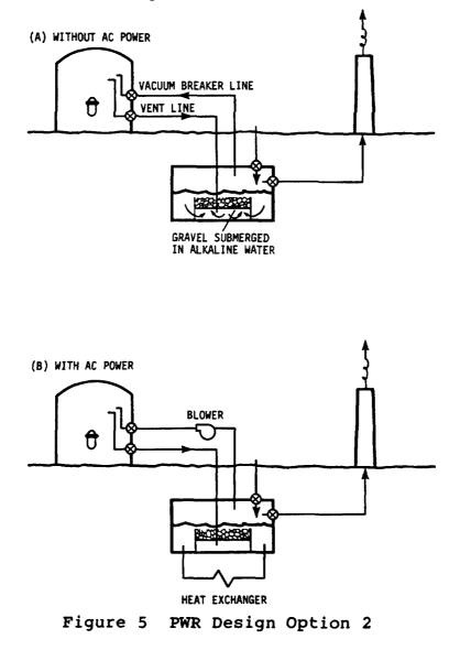
submerged in an alkaline water pool. This option has the capability to condense steam, which option 1 does not. Estimated fission product removal efficiencies are: 98% particles, 98% I<sub>2</sub>, 50% CH<sub>3</sub>I, 0% Xe and 0% Kr. In this option a provision for re- circulation of the filtered containment exhaust and long term heat removal from the suppression pool has been made.
