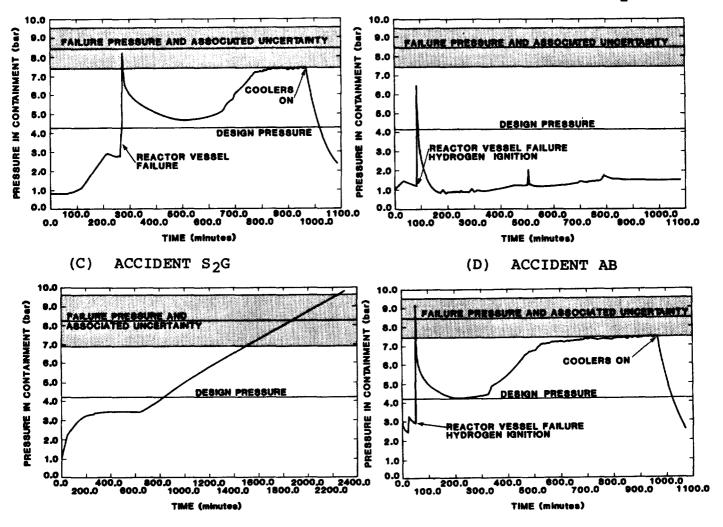
Figure 1 MARCH Code Calculations of Containment Pressure Versus Time for Four Hypothesized Accidents in the Baseline PWR Plant
