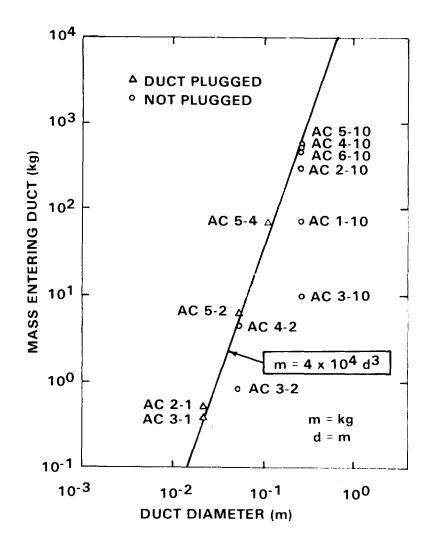
FIGURE 6. Duct Plugging as a Function of Duct Diameter. (Neg. 801843-4)
