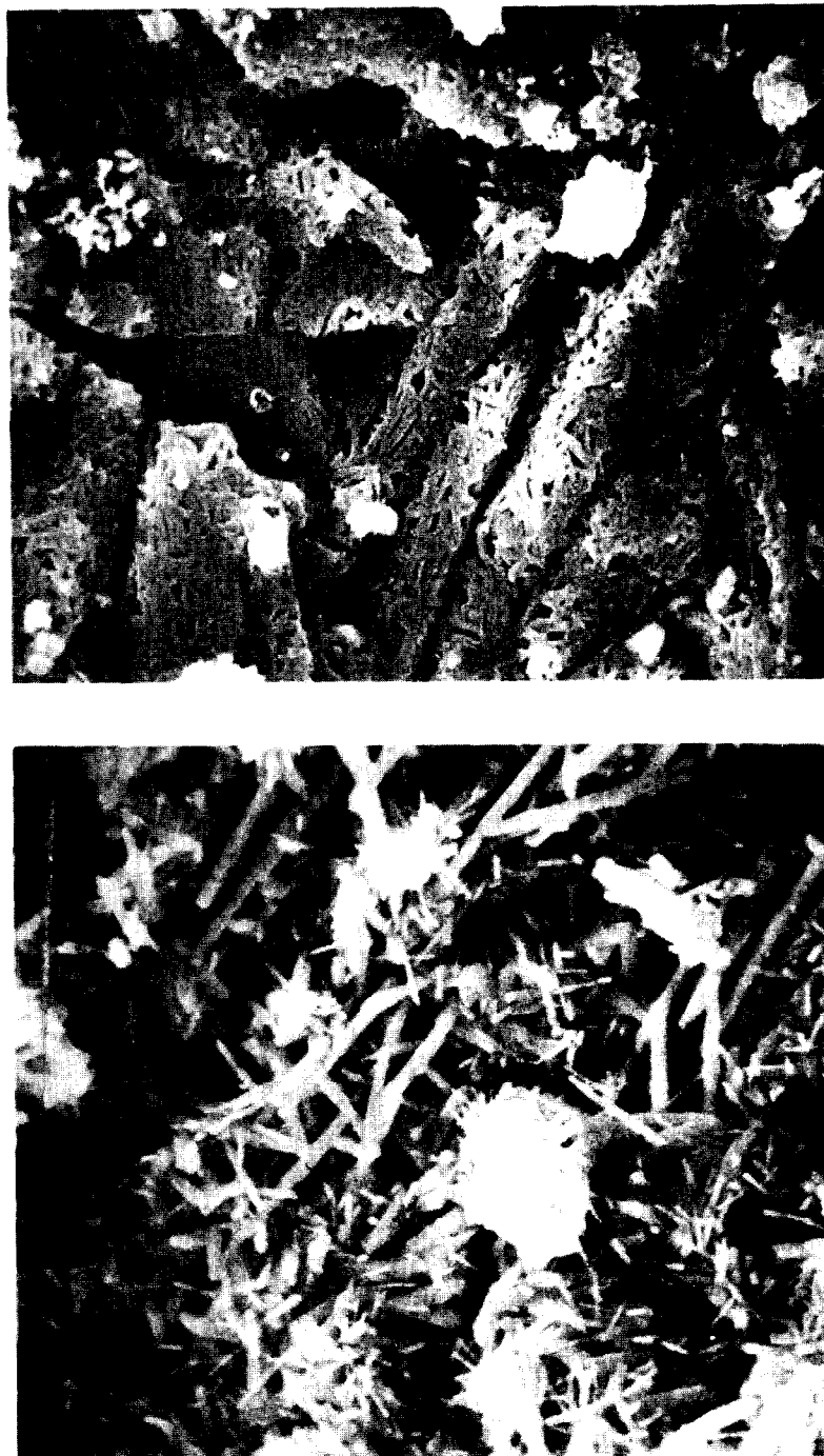
Fig. 2. Scanning electron micrographs of a flake of commercial \text{Ba}(\text{OH})_2 \cdot 8\text{H}_2\text{O} (top) and the \text{BaCO}_3 product. The product was obtained at a process humidity <60\% (original photo, 8.9 \times 11.4 cm; magnification, 5000\times ).
