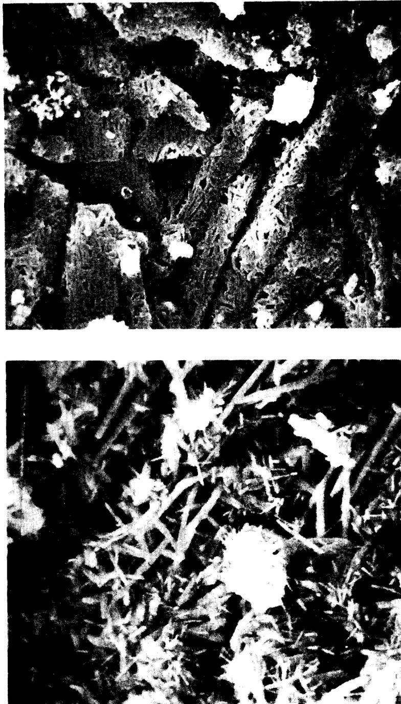
Fig. 2. Scanning electron micrographs of a flake of commercial  $\text{Ba(OH)}_2 \cdot 8\text{H}_2\text{O}$  (top) and the  $\text{BaCO}_3$  product. The product was obtained at a process humidity  $<60\%$  (original photo,  $8.9 \times 11.4$  cm; magnification,  $5000\times$ ).
