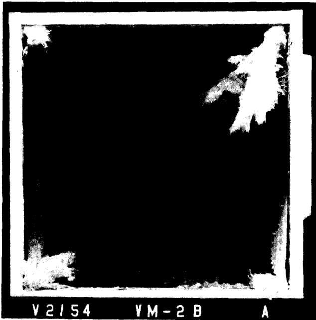
Figure 7: Typical failure of a metal frame filter
