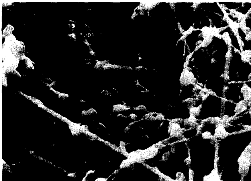
Figure 6: Scanning electron micrograph of a filter paper loaded with polystyrene latex aerosols
