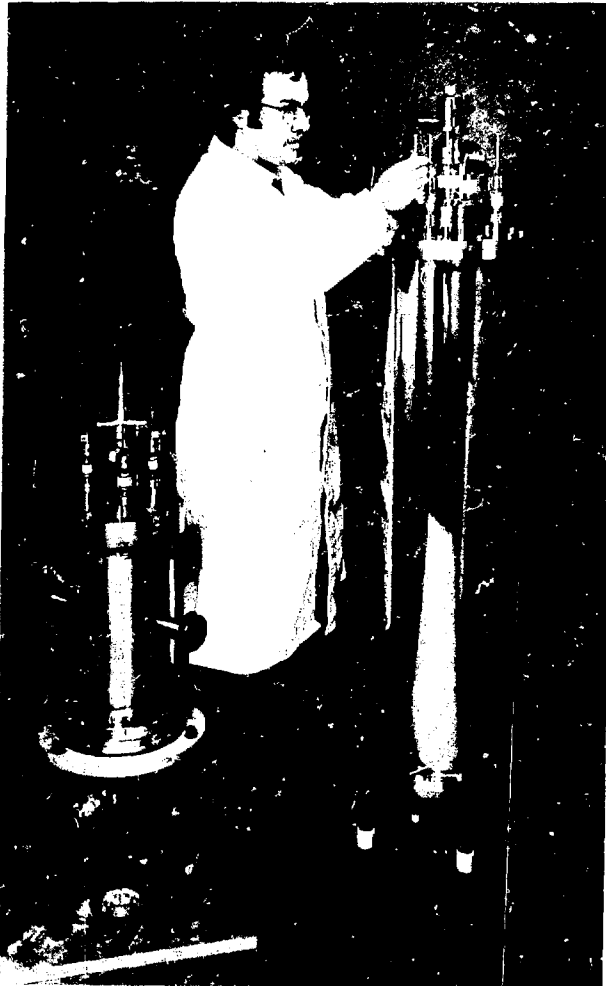
Figure 3 Photograph of two experimental vessels. Small vessel for materials tests and 50 litre vessel.
