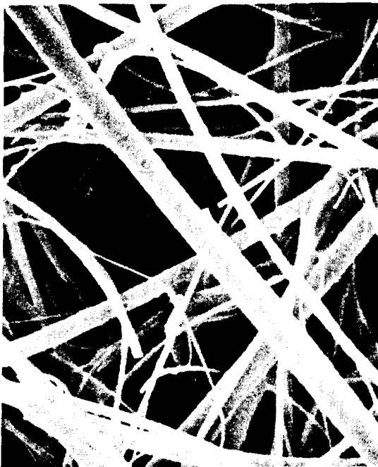
Figure 11. Material type 1 after exposure to condensed steam for 2 h.
