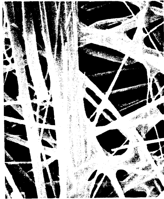
Figure 12. Material type 1 after exposure to an air steam mixture 85 % RH at 85°C for 2 h.
