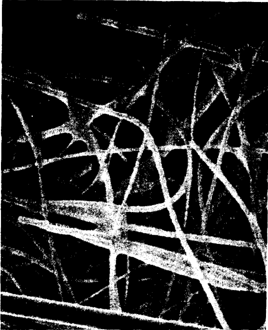
Figure 9. Reference Specimen, new filter material, type 1. Magnification x 2 000.
