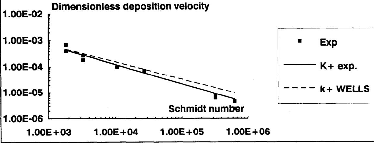
**Figure 2: Dimensionless deposition velocity of large particles for turbulent flow conditions**
