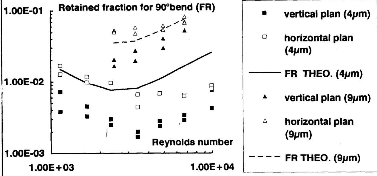
Figure 6: Particles deposition in the overall line versus Reynolds number
