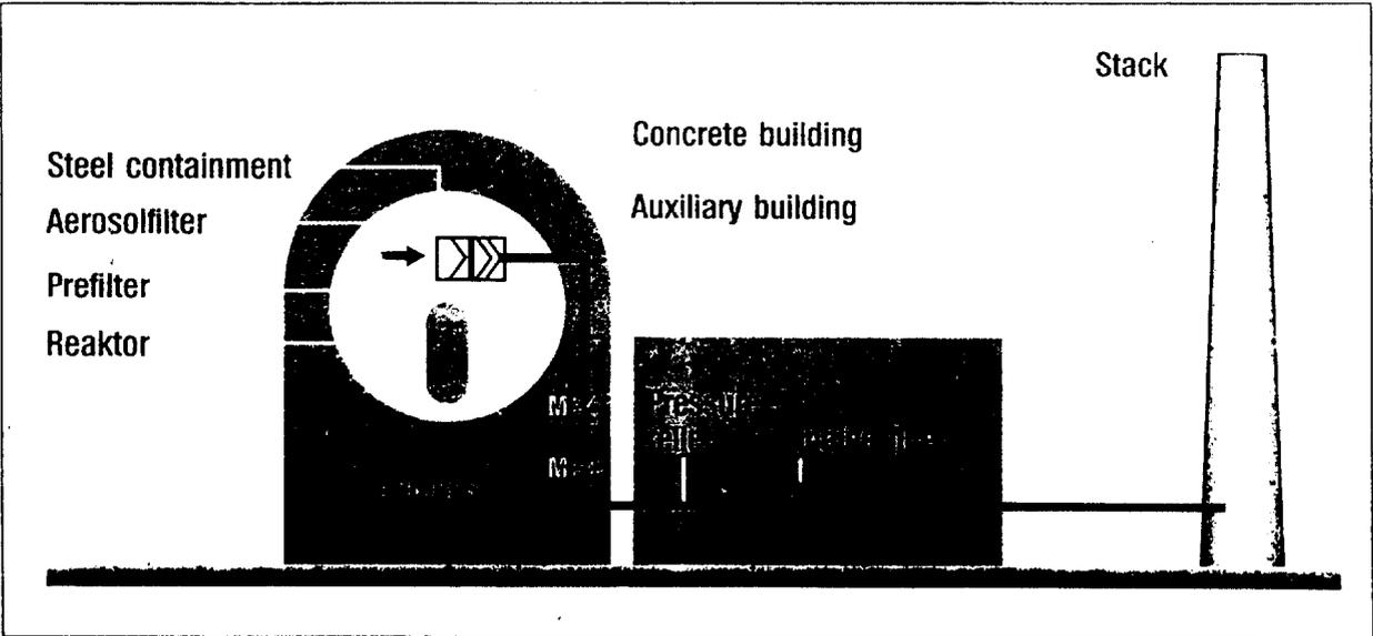
Figure 2: Two options for arranging prefilters and aerosol filters in pressurized water reactors
