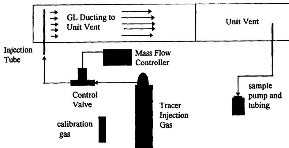
Figure 10 Tracer gas injection setup
