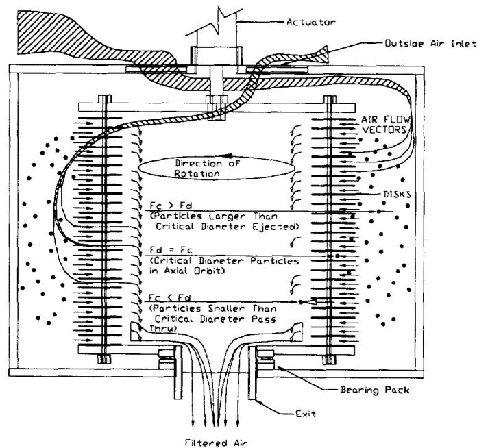
**Figure 1. Schematic Representation of the BLMT Filter**
