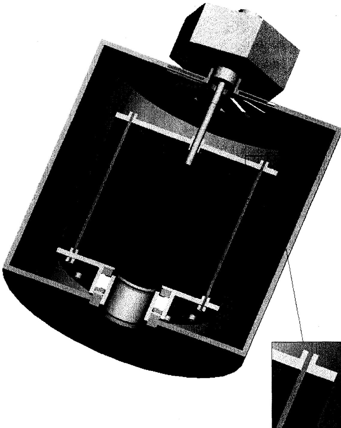
**Figure 3 Cut-Away CAD Rendering of the BLMT Filter**
