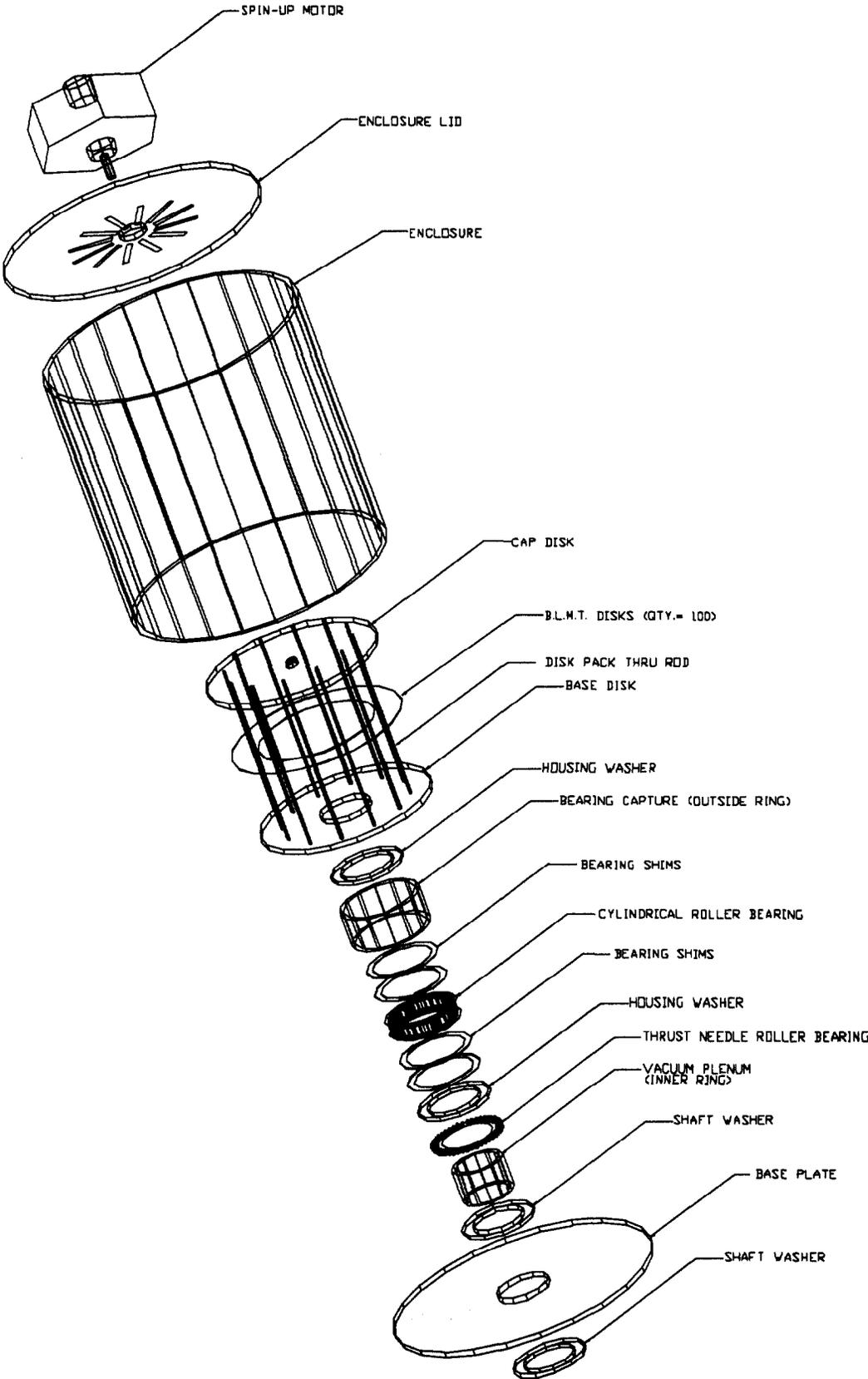
Figure 2 Exploded View of the BLMT Filter
