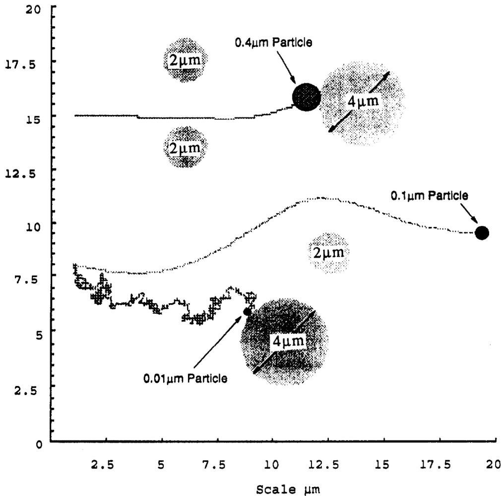
Figure 6 Trajectories of three different diameter particles through the fiber matrix in Figure 2. Particle diameters were selected to illustrate conventional mechanical collection mechanisms:  $0.01\mu\text{m}$  for Brownian motion,  $0.1\mu\text{m}$  for interception, and  $0.4\mu\text{m}$  for inertia.
