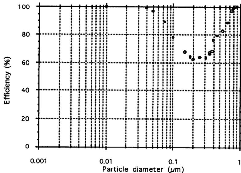
Figure 11 Filter efficiency computed for different particle diameters (density 1 g/cm<sup>3</sup>) through the staggered hexagonal array in Figure 3 with a uniform inlet air velocity of 3 cm/s. The pressure drop across the fiber matrix element is  $3.2 \times 10^{-5}$  inches of water.
