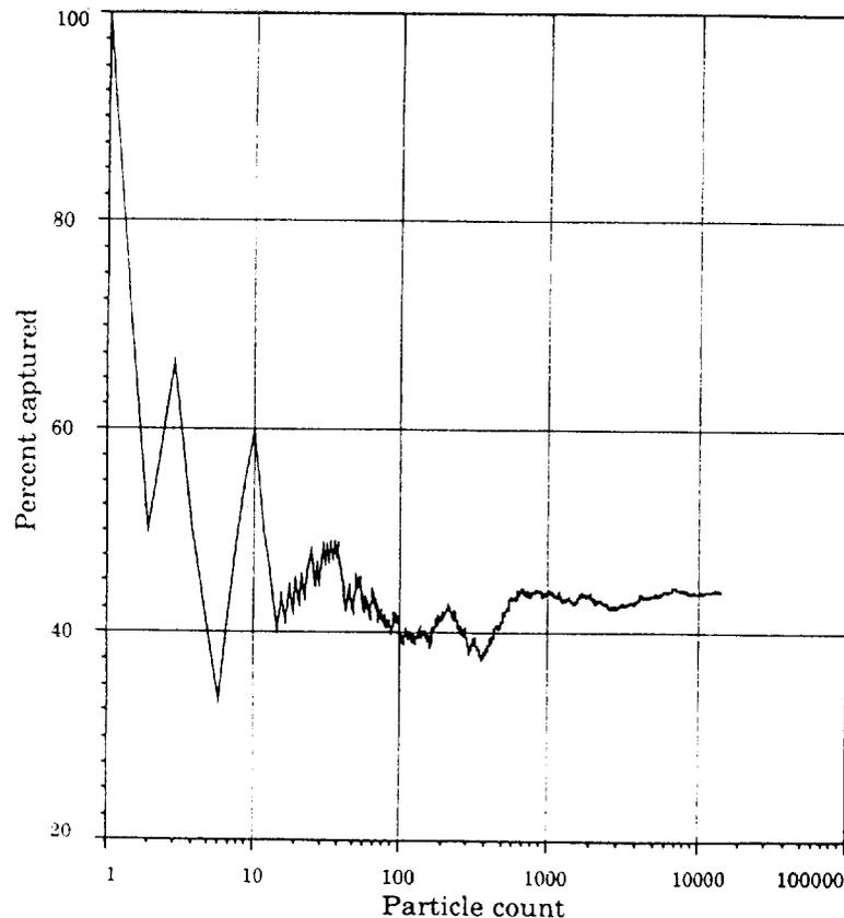
Figure 8 Cumulative efficiency of increasing number of  $0.3\mu\text{m}$  diameter particles (density  $1\text{ g/cm}^3$ ) passing through the crossed fiber matrix in Figure 4 with a uniform inlet air velocity of  $20\text{ cm/s}$ .
