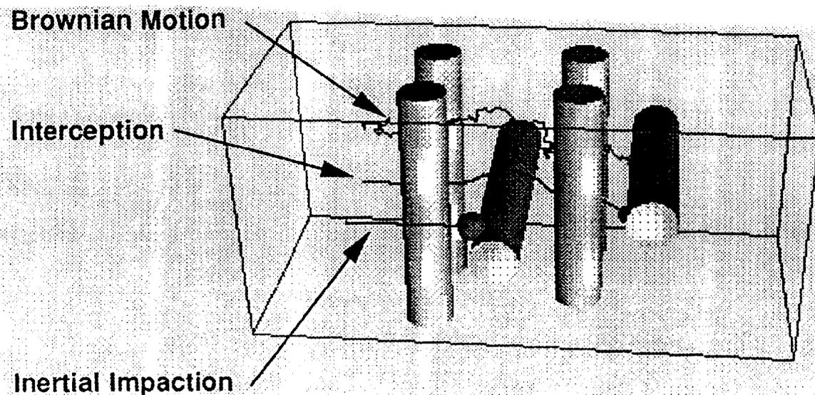
Figure 7 Trajectories of three different diameter particles through the fiber matrix shown in Figure 4 with the inlet air velocity at 20 cm/s. The diameter of the particles were selected to illustrate the conventional collection mechanisms due to Brownian motion, interception and inertial impaction. Note that the particle sizes are not to scale to allow visualization.
