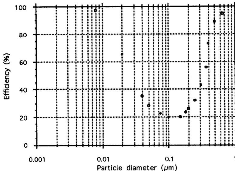
Figure 9 Filter efficiency computed for different particle diameters (density 1 g/cm<sup>3</sup>) passing through the crossed fiber matrix in Figure 4 with uniform inlet air velocity of 20 cm/s. The pressure drop across the fiber matrix element is  $4.4 \times 10^{-5}$  inches of water.
