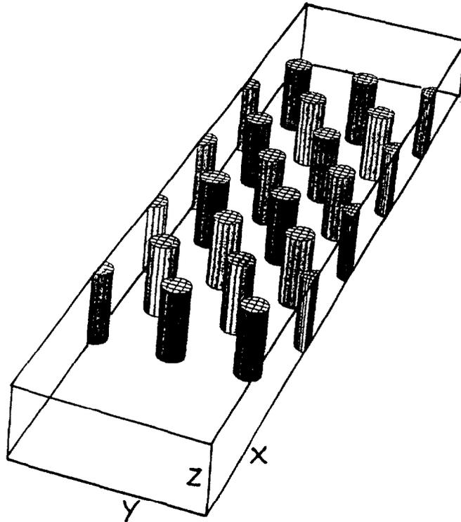
Figure 3 3-D fiber matrix with  $1\mu\text{m}$  diameter fibers arranged in a staggered hexagonal array. The fiber matrix  $L \times W \times H$  is  $23.0\mu\text{m} \times 6.5\mu\text{m} \times 5.0\mu\text{m}$ . The fiber volume fraction is 0.0825, and air flow is in X direction.
