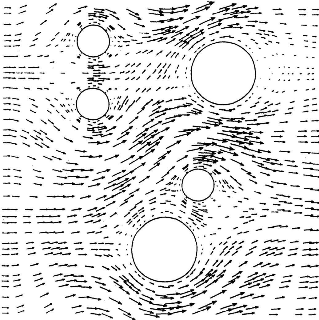
Figure 2 Air velocity vector field through 2-D fiber matrix at  $20\text{ cm/s}$  initial velocity. The fiber matrix is  $20\mu\text{m} \times 20\mu\text{m}$  with  $2\mu\text{m}$  and  $4\mu\text{m}$  diameter fibers. The fiber volume fraction is 0.0864.
