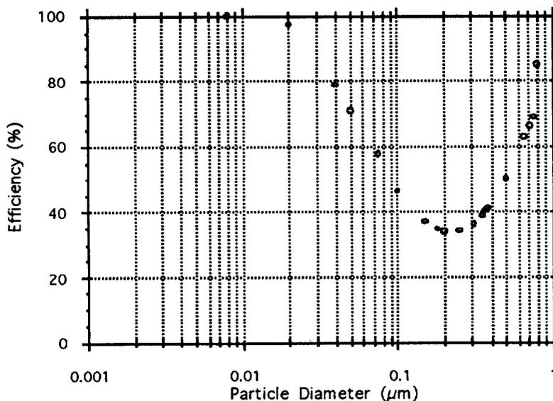
Figure 10 Filter efficiency computed for different particle diameters (density 1 g/cm<sup>3</sup>) through the crossed fiber matrix in Figure 4 with a uniform inlet air velocity of 20 cm/s. The pressure drop across the fiber matrix element is  $4.4 \times 10^{-6}$  inches of water.
