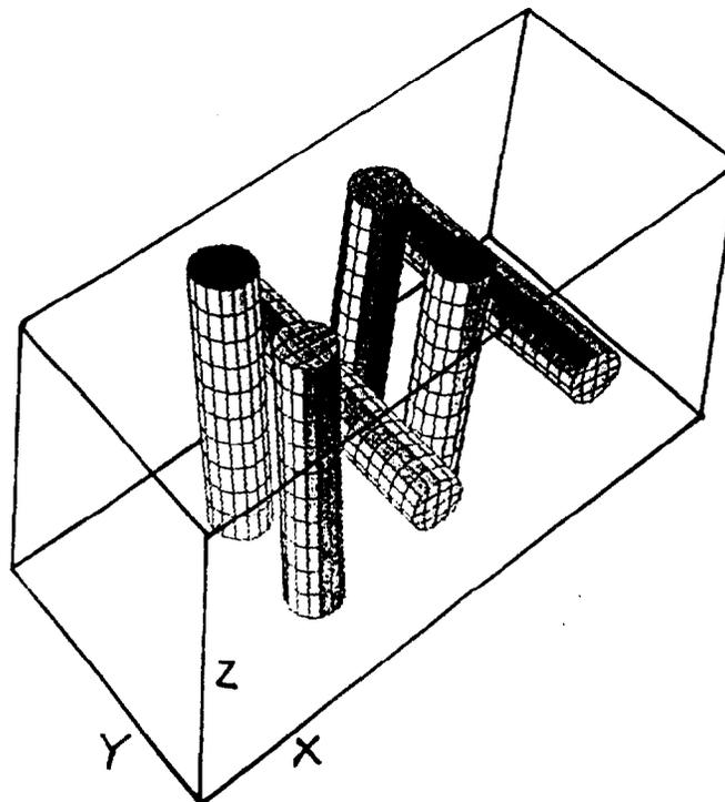
Figure 4 3-D fiber matrix with  $1\mu\text{m}$  fibers arranged in a crossed fiber array. The fiber matrix  $L \times W \times H$  is  $11\mu\text{m} \times 5\mu\text{m} \times 5\mu\text{m}$ . The fiber volume fraction is 0.0843 and air flow is in X direction.
