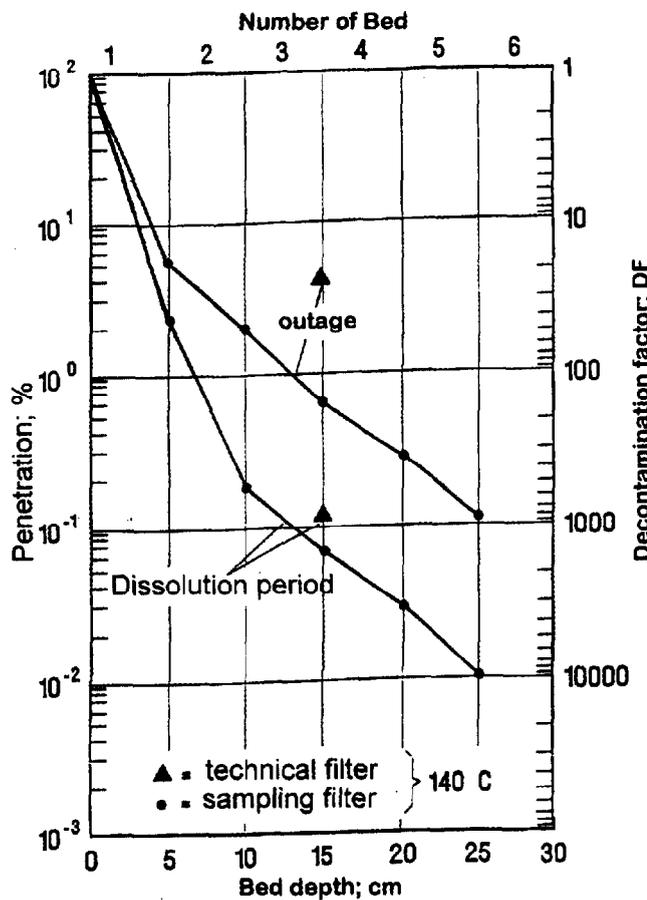
The decontamination factors obtained with the small scale columns (sampling filter: inner diameter 0.032 m, bed depth 0.15 m) and the technical iodine filter (annular cylinder with a bed depth of 0.15 m), are traced in figure 2. The small scale filters reveal a higher iodine removal performance than the technical iodine filter. These values result from 12 measuring periods between 1989 and 1991.
