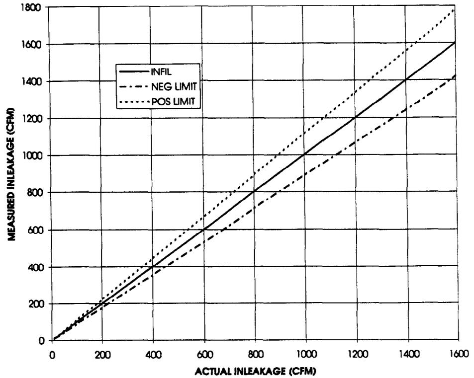
Figure 5. Unfiltered Inleakage no Makeup-Case V
