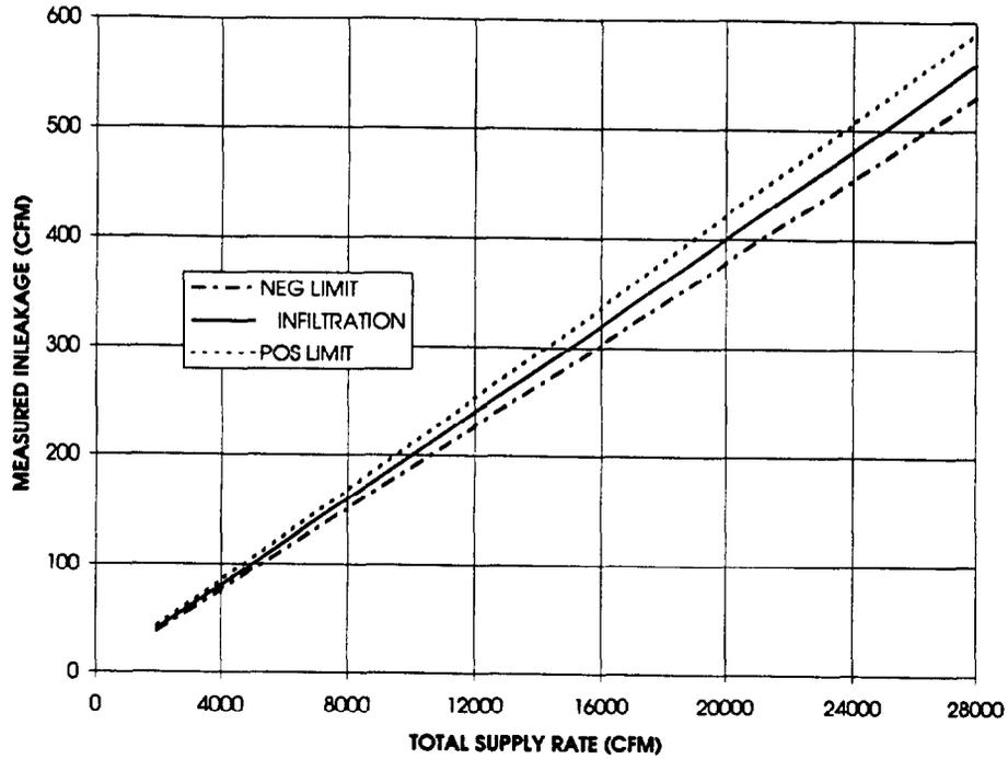
Figure 11. Minimum Measurable Inleakage, dC=0.01, dQ=0.05
