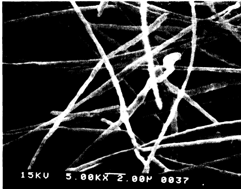
Figure 12. Electron micrograph of the steel fiber media made from 0.5 \mu\text{m} steel fibers.
