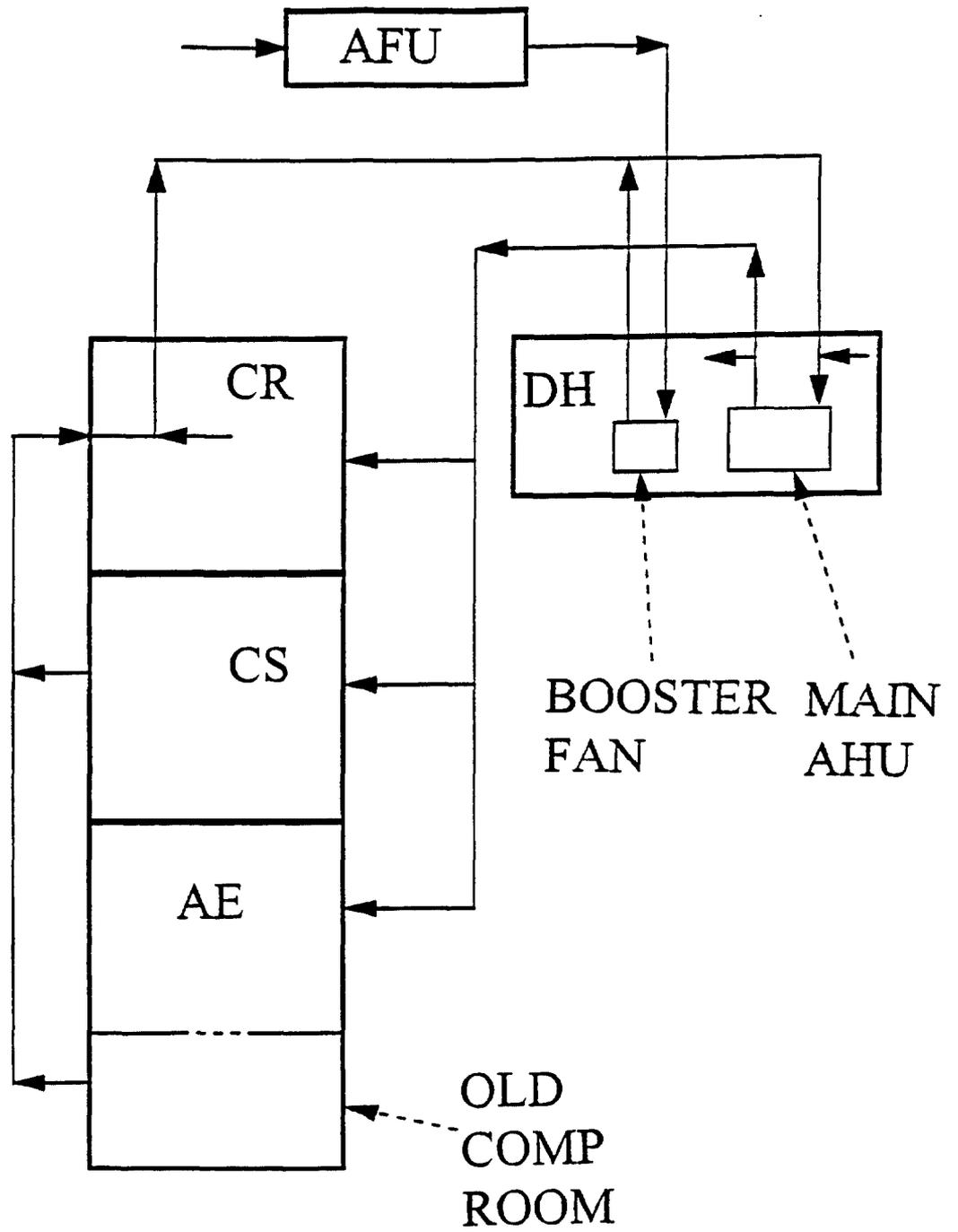
Figure 3. Quad Cities B Train CRE Emergency Ventilation System
