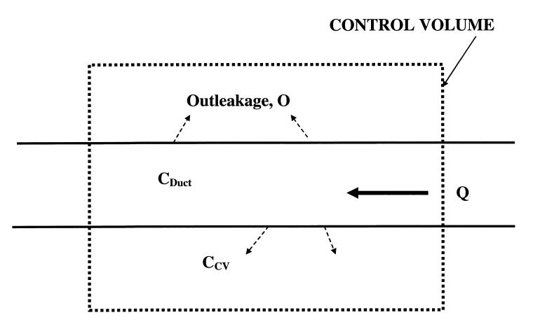
Figure 9. Non-CREVS Component Leakage Test
