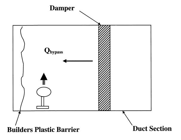
Figure 8. Duct Outleakage Test
