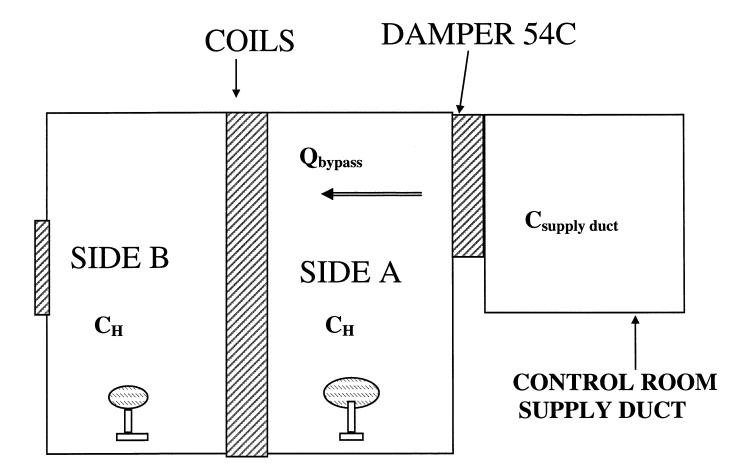
Figure 7. Damper Leakage by Tracer Decay Method
