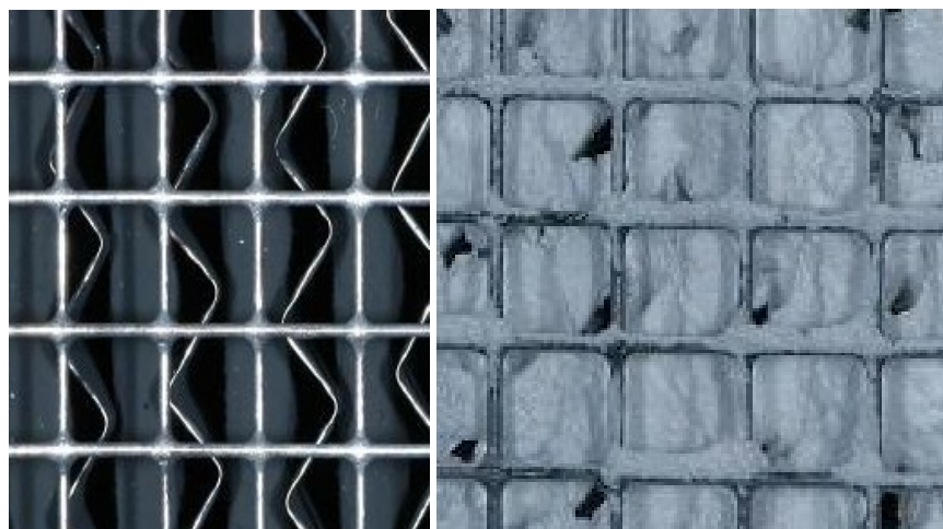
Figure 13. Photos of the front surfaces of HEPA filter that has been with soot (left) and KCl (right). Each filter has been loaded to six inches wc differential pressure.
