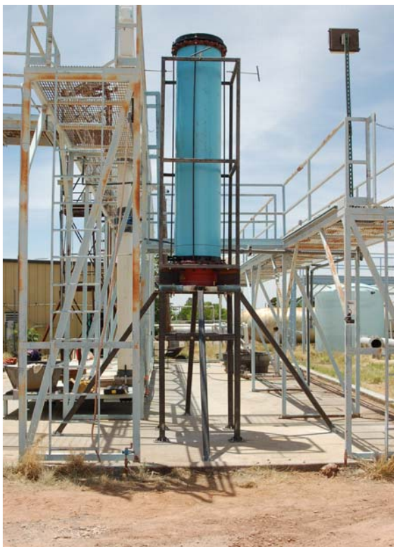
Figure 5: Side view of prototype full-scale rig for qualification of 610-mm x 610-mm x 292-mm (12-in x 12-in x 11 1/2 -in) high-strength filters to pressure impulse test, less test section. (left)
