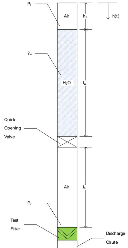
**Figure 1:** Schematic of falling water column concept for qualification testing of high-strength nuclear-grade HEPA filters<sup>(3)</sup>.
