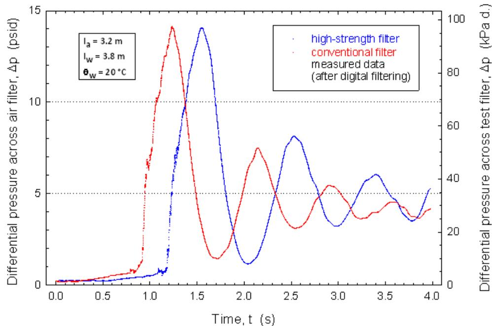
Figure 2: Plots of differential pressure across a 203-mm x 203-mm x 149-mm (8-in x 8-in x 5<sup>7</sup>/<sub>8</sub>-in) conventional, and a prototype, high-strength filter during a pressure-impulse test<sup>(8)</sup>.
