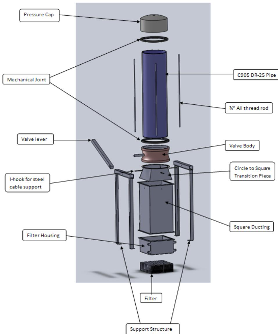
Figure 3: Exploded view of preliminary design of full-scale prototype test rig for qualification testing of high-strength filters.
