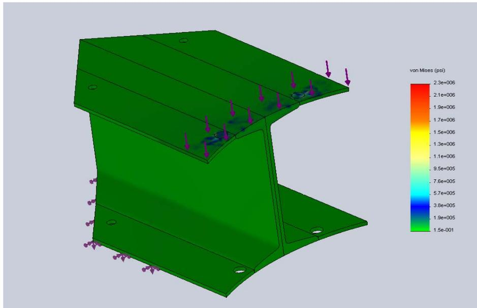
Figure A-1: Stress distribution on top-surface of edge on valve support member at eight-times actual load (typ. one of four).
