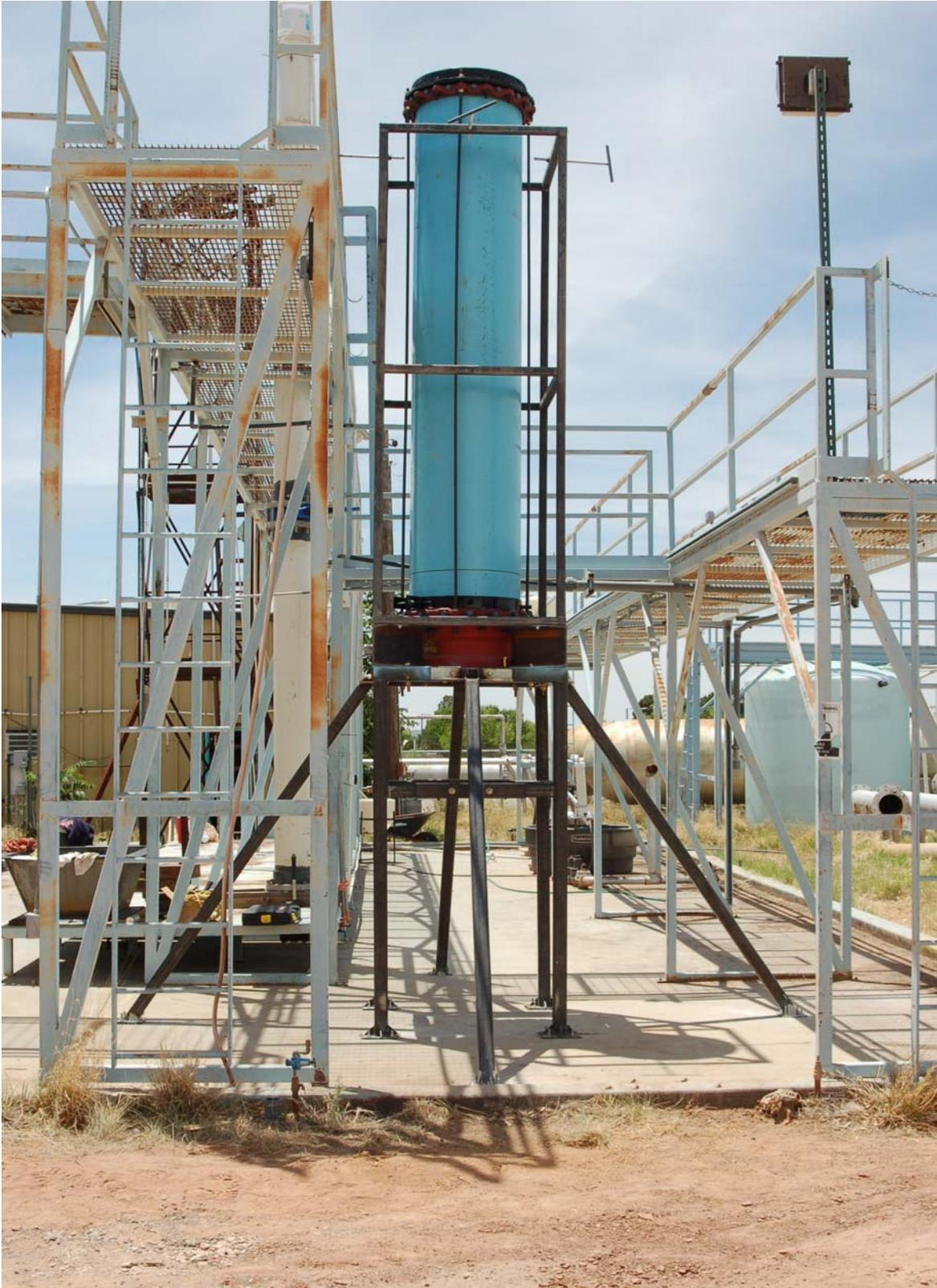
Figure A-2: Side view of assembled prototype full-scale rig for qualification of 610-mm x 610-mm x 292-mm (12-in x 12-in x 11<sup>1</sup>/<sub>2</sub>-in) high-strength filters to pressure impulse test, less test section.
