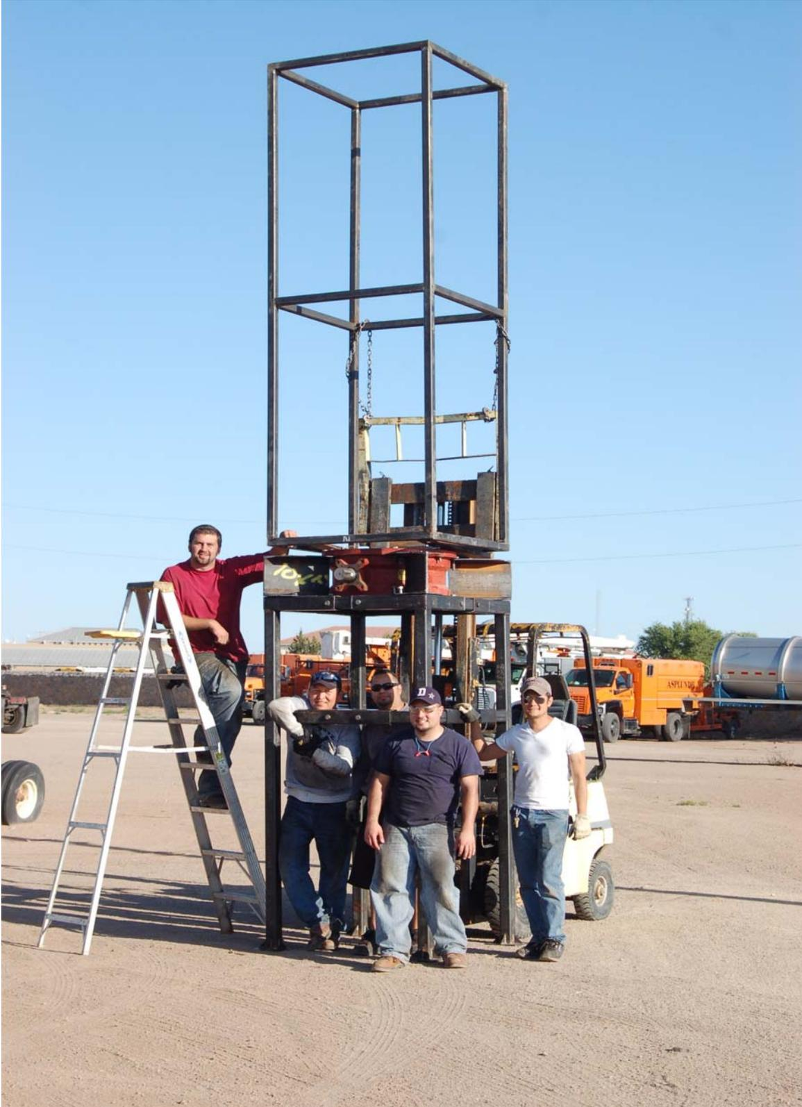
Figure A-3: First assembly of valve and upper pipe-enclosure cage on support structure (with design team).
