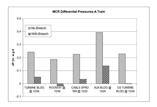
Figure 3. Differential Pressures for two Inleakage Tests
