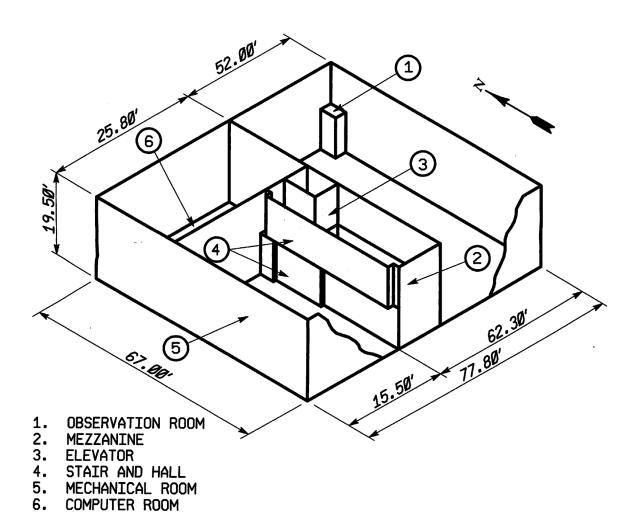
Figure 2. Control Room Envelope at Fort Calhoun Station.
