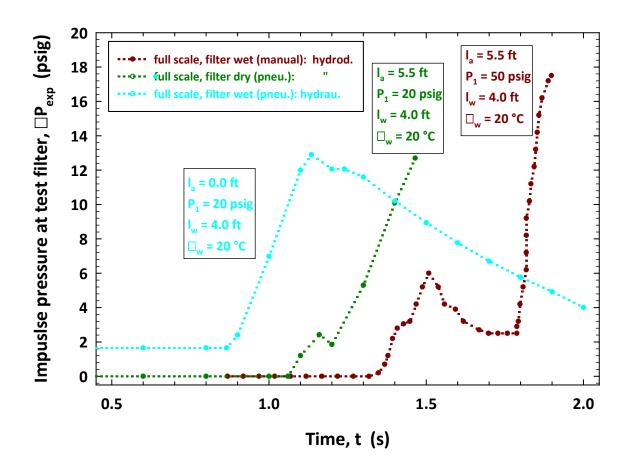
Comparison of test results for <u>propelled</u> to those of <u>falling</u> water column
