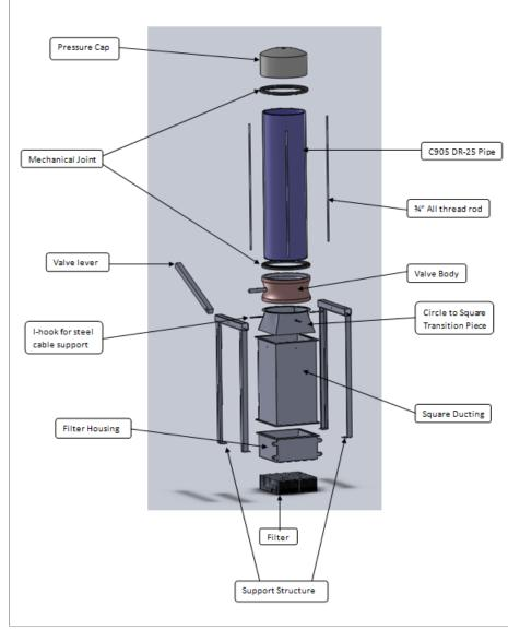
Assembly rendering for preexisting prototype test rig
