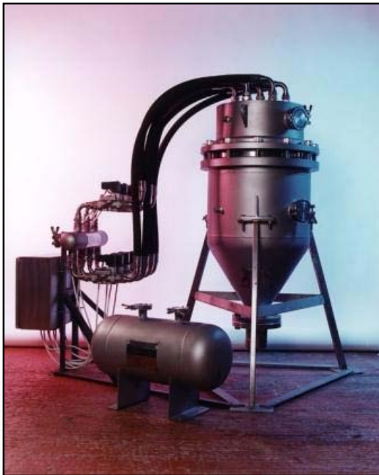
Glovebox pulsed jet MOX pellet grinding coolant (Air) filter for BelgoNucleaire
