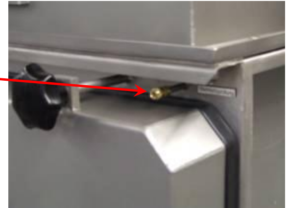
Filter gasket leak test port (HEPA-filter)
