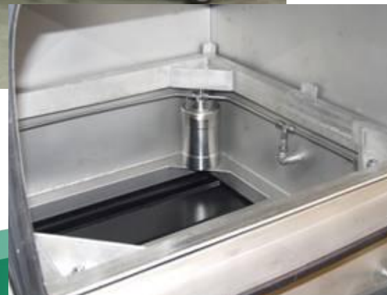
Pneumatic filter declamping device for activated carbon - & HEPA-filter
