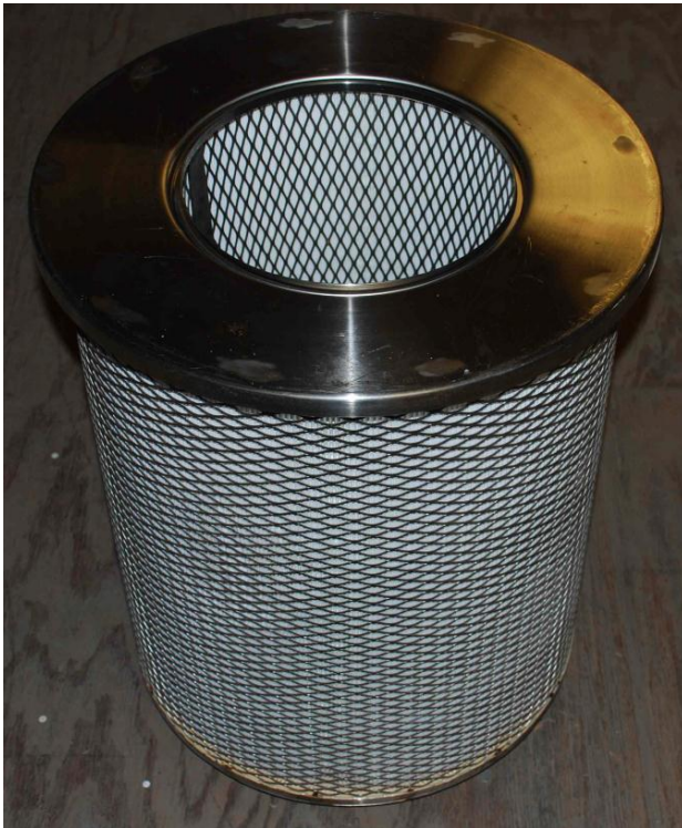
Photo of a Remote Change HEPA filter design
