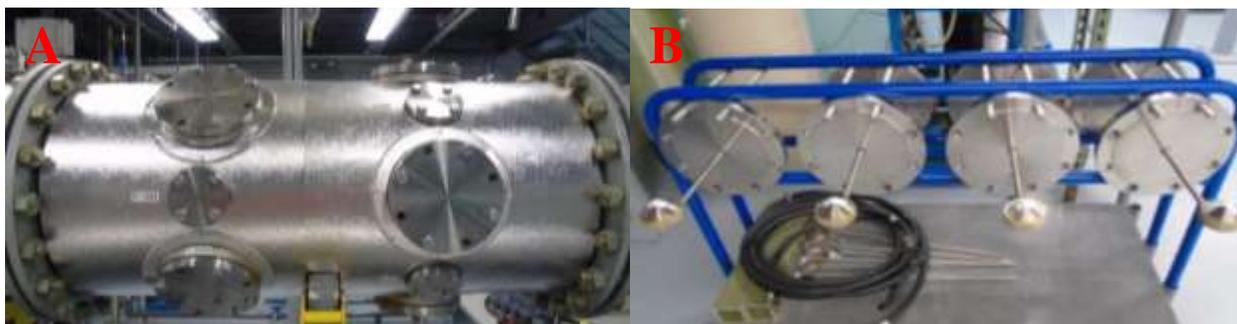
**Figure 13.** A.) In-duct coupon and Pilat Impactor sampling section of the RLSTS. B.) In-duct coupon samplers.
