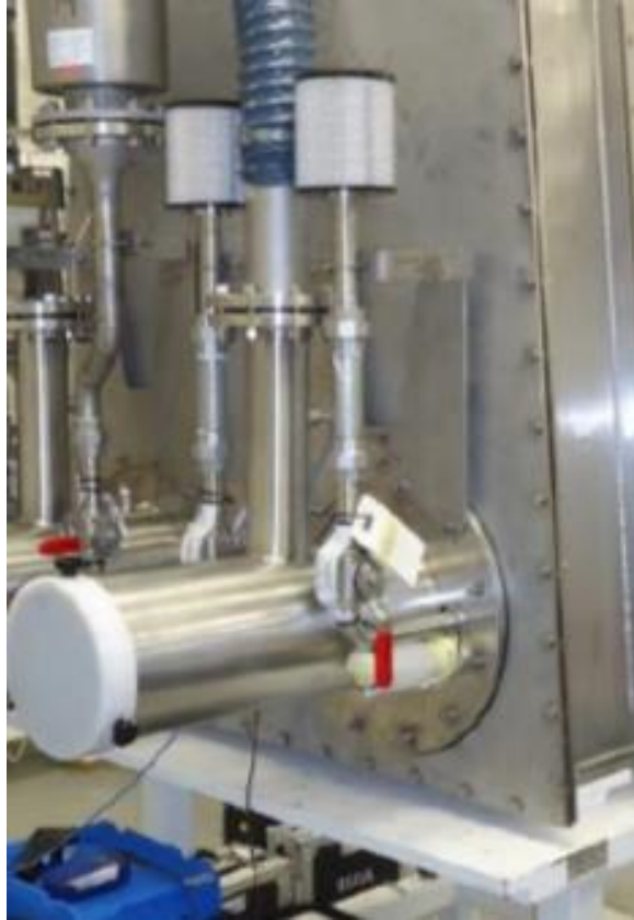
Figure 15 - Standard VXA with 6l/s control port filters [17]
