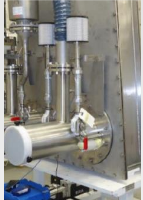
Company Standard VXA fitted to glove box
