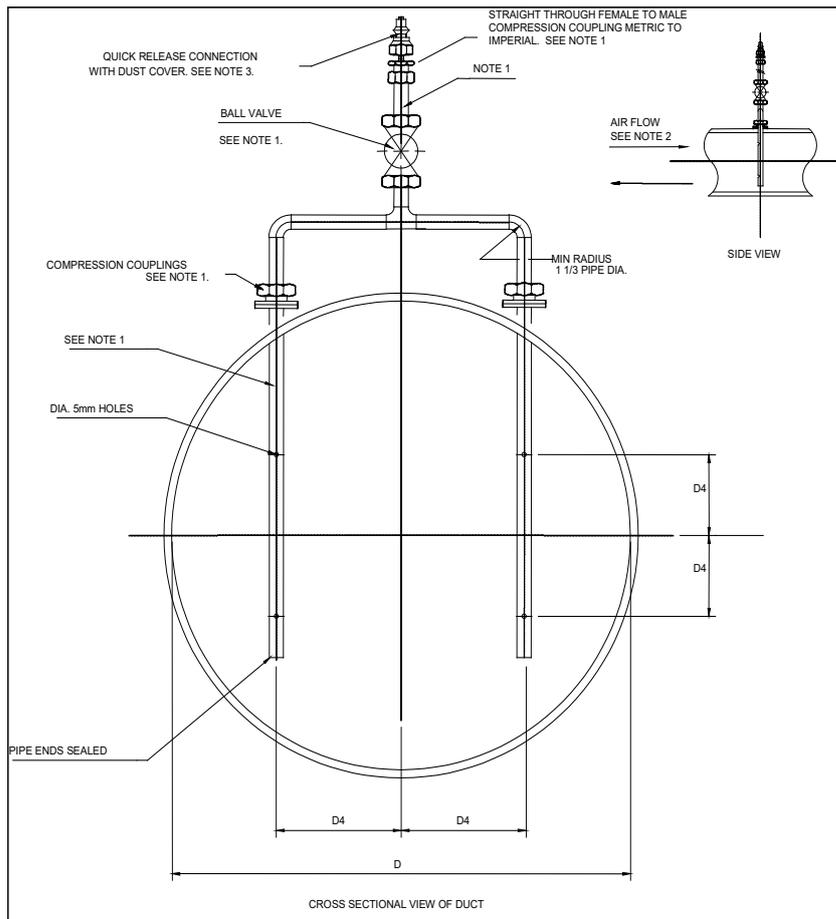
**Fig 16, Typical 4 Hole Probe Array For Circular Ducts**
