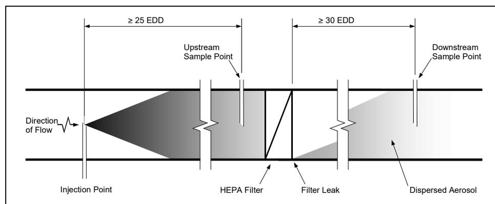
The particulate challenge commonly used is a Dispersed Oil Particulate, most commonly known by its initials DOP. With DOP testing within the UK the particulate challenge is a light mineral oil which is thermally vaporised in the presence of CO<sub>2</sub> and condenses to form a uniform particulate challenge of oil droplets of around 0.3µm diameter. The abatement HEPA filters used in UK Nuclear Facilities normally have
