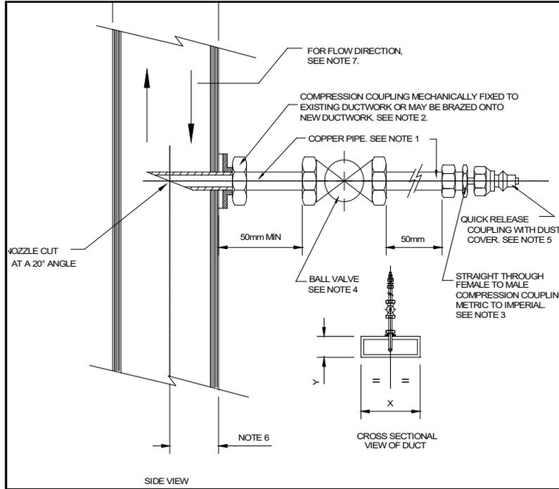
**Fig 14. Typical Single Probe**
