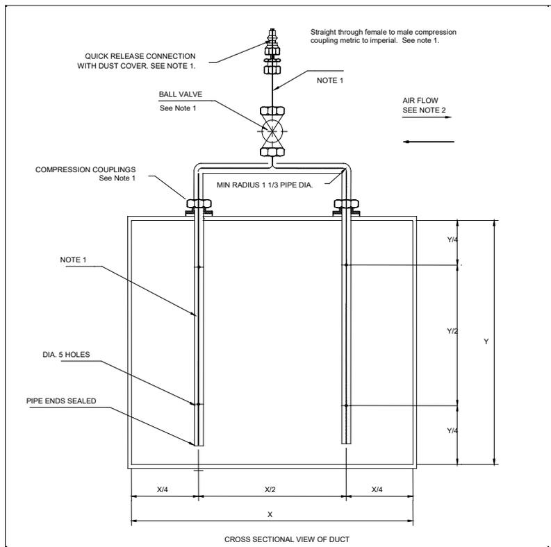
**Fig 15, Typical 4 Hole Probe Array For Rectangular Ducts**
