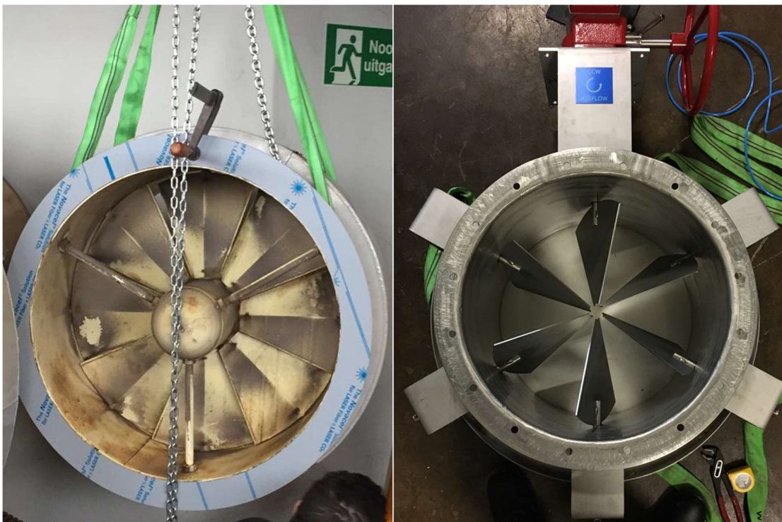
Figure 5 Original IVD on the left with center hub and new IVD on the right with center opening
