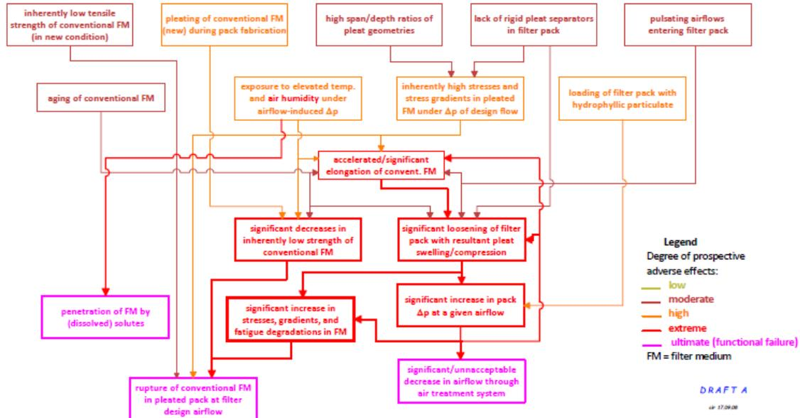
**Figure A:** Prospective mechanisms and relationships underlying functional failure of radial-flow HEPA filters (without rigid pleat separators) having an unreinforced, filter medium in an aged, non-water repellent, fatigued, and particle-loaded condition, during operation in their service locations.
