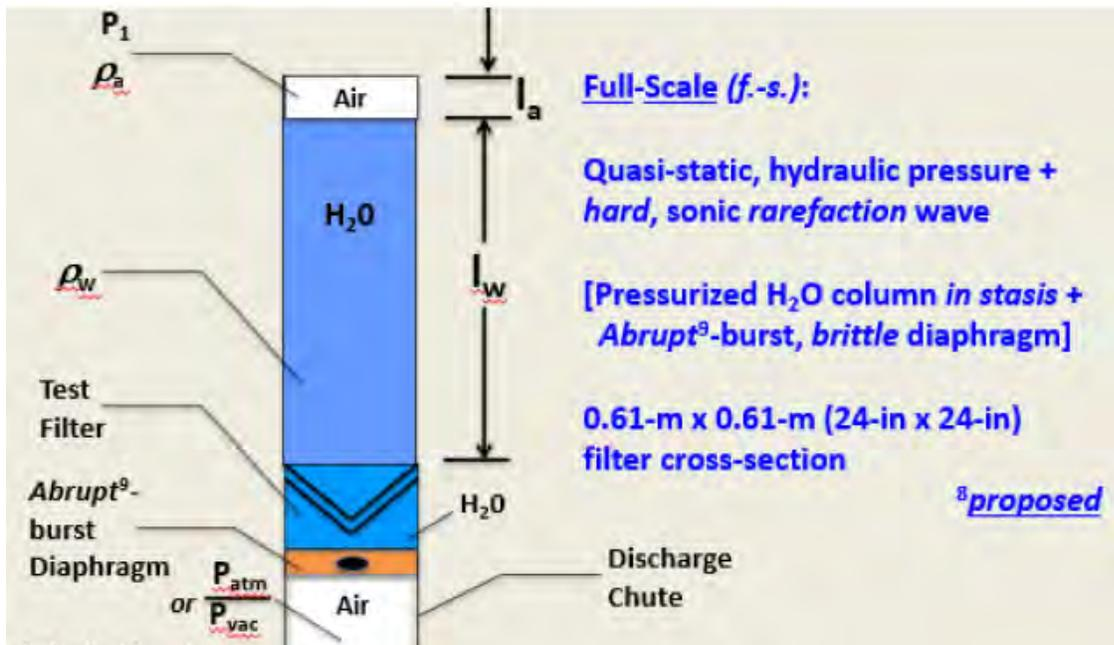
**Figure D:** Schematic of proposed resistance-to-pressure impulse test stand based upon the quick release of a pressurized water column initially *in stasis*, toward qualification of nuclear-grade HEPA filters. Simplification of dynamically pressurized H<sub>2</sub>O column of [15].
