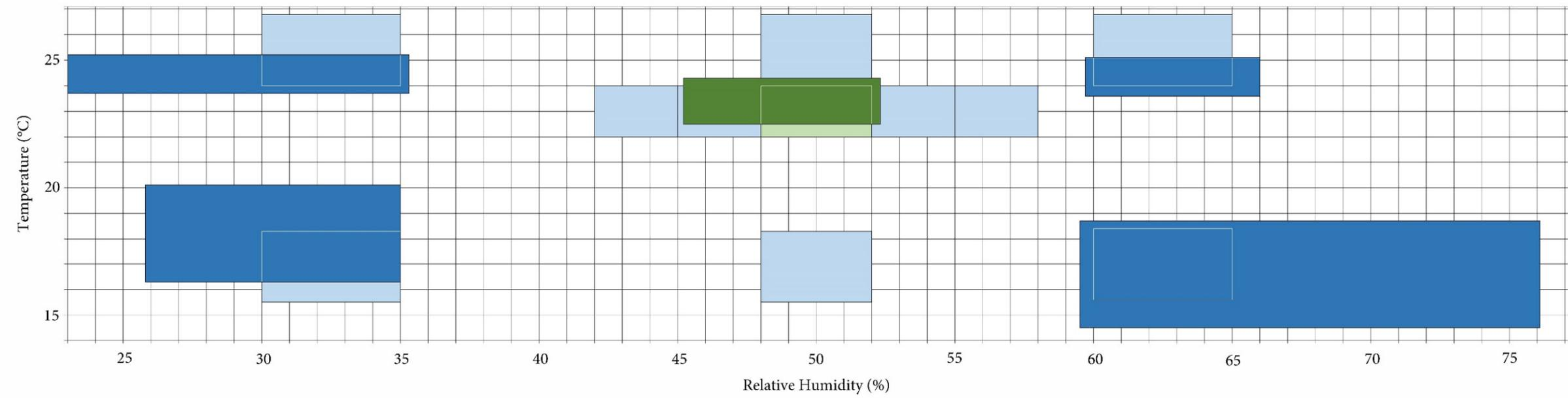
Figure A3. Actual conditions experienced during preliminary study (dark) overlaid on target ranges for conditioning and testing environments (light).
