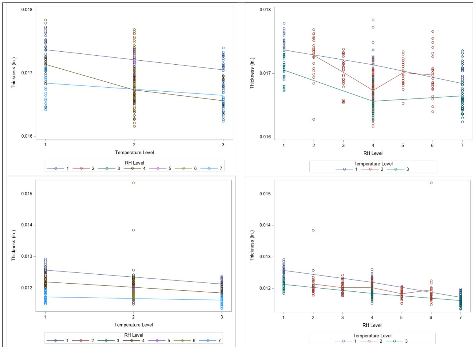
Figure 9. RH and temperature interaction plots for thickness for M008 (top) and A114 (bottom).
