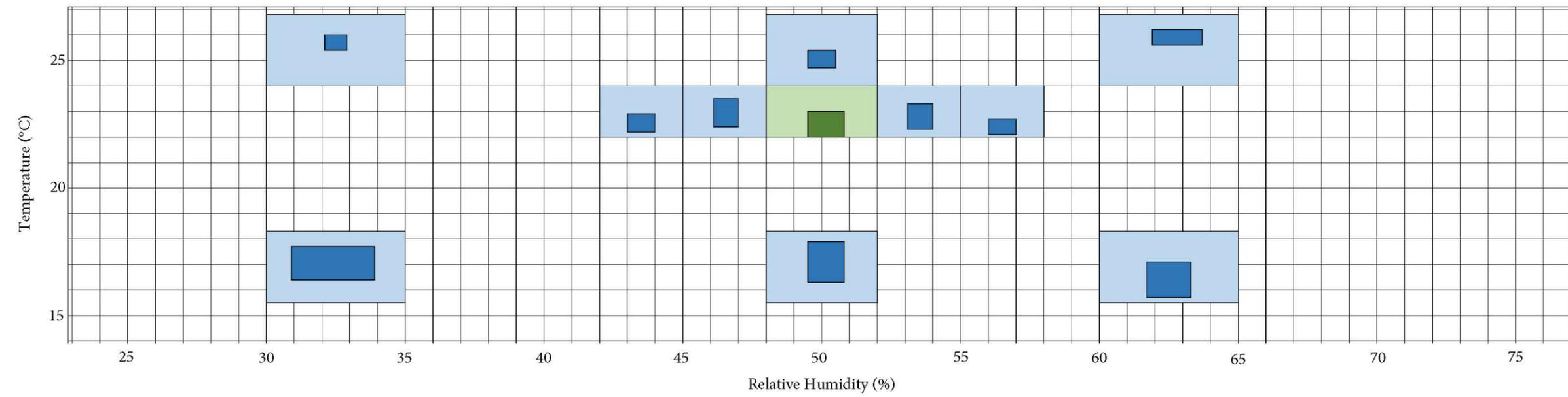
Figure A2. Actual conditions experienced during the Effect of Testing Environment Conditions Study (dark) overlaid on target ranges for conditioning and testing environments (light).
