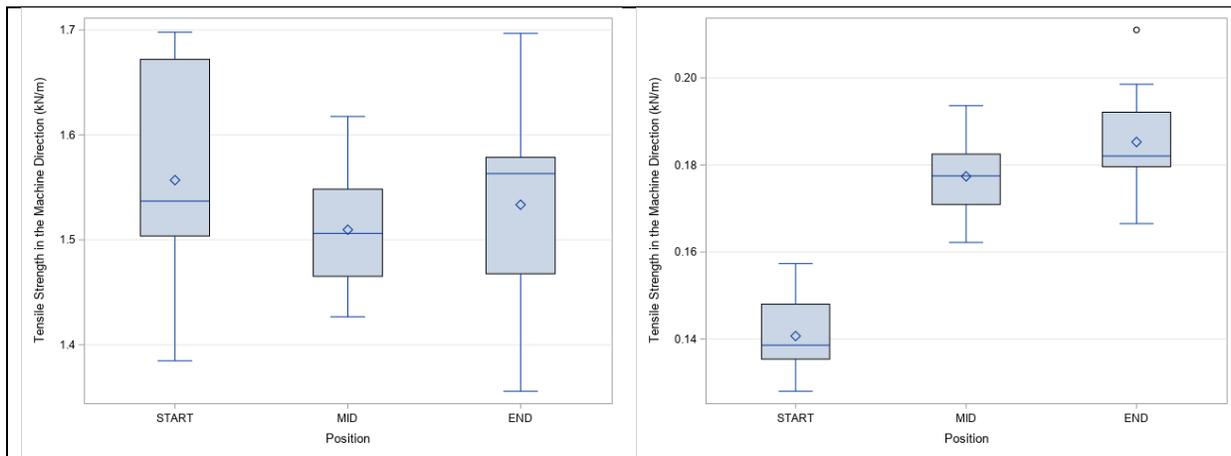
Figure 2. Distribution plots for tensile strength in the machine direction with respect to position for M008 (left) and A114 (right).
