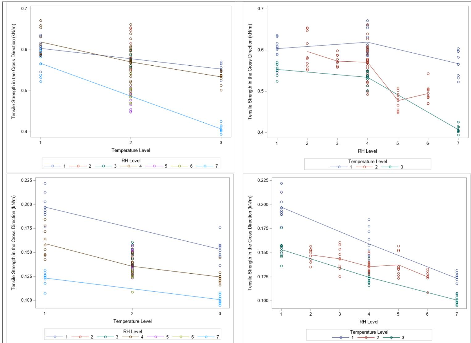
Figure 7. RH and temperature interaction plots for tensile strength in the cross direction for M008 (top) and A114 (bottom).
