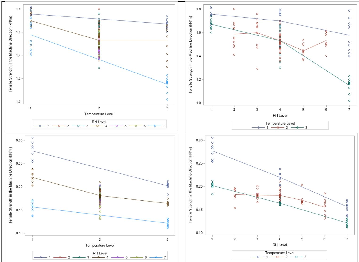
Figure 6. RH and temperature interaction plots for tensile strength in the machine direction for M008 (top) and A114 (bottom).
