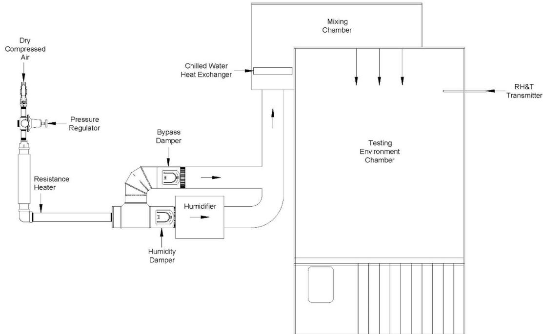
Figure 1. Schematic of Testing Environment Chamber.
