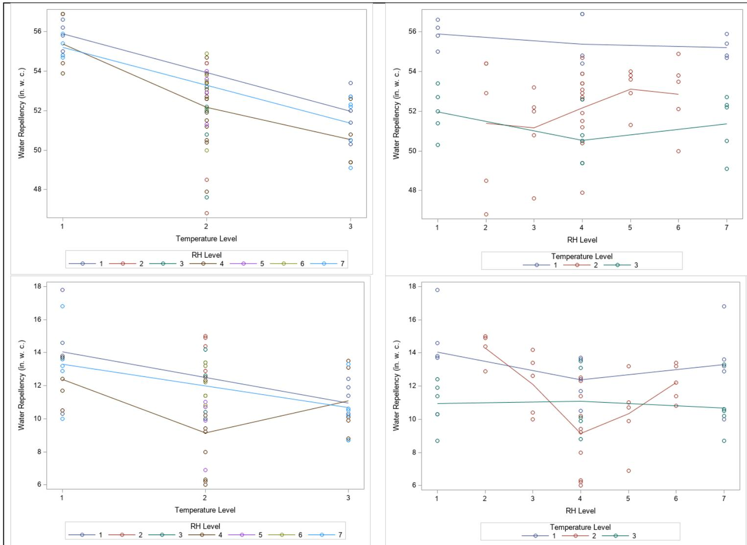
Figure 8. RH and temperature interaction plots for water repellency for M008 (top) and A114 (bottom).
