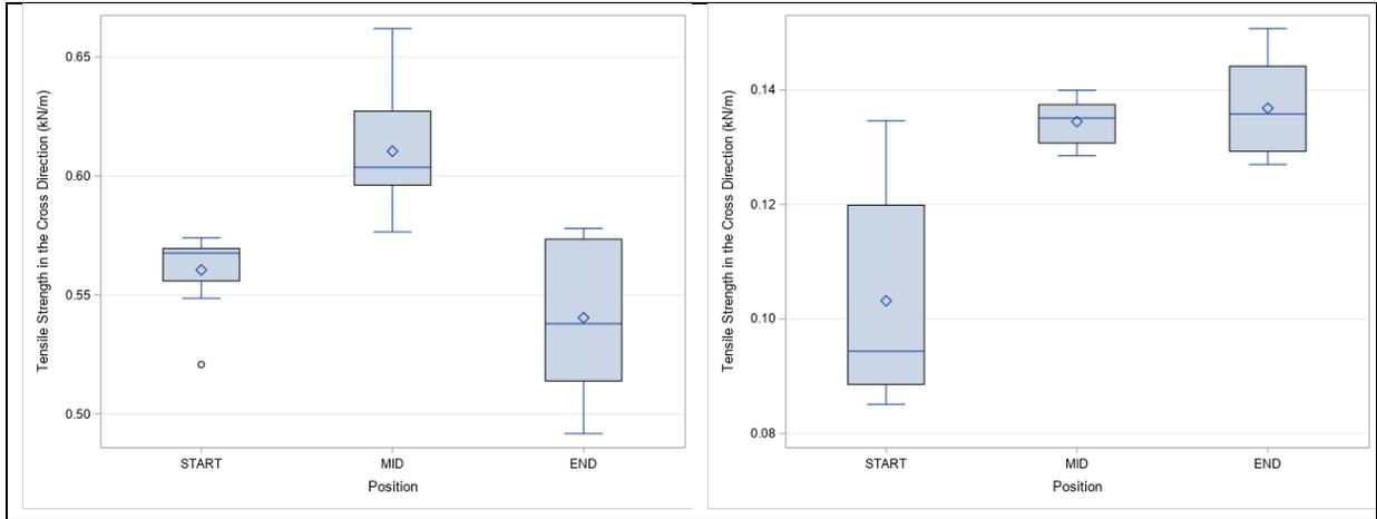
Figure 3. Distribution plots for tensile strength in the cross direction with respect to position for M008 (left) and A114 (right).
