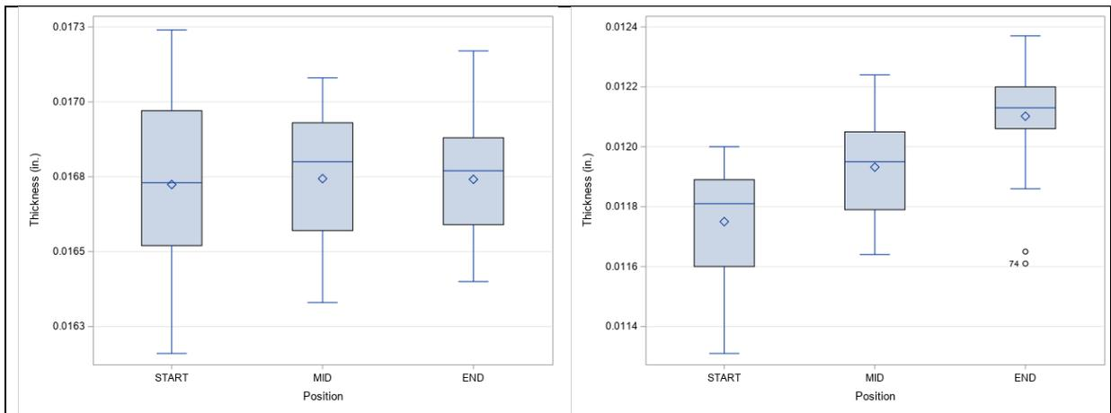
Figure 5. Distribution plots for thickness with respect to position for M008 (left) and A114 (right).
