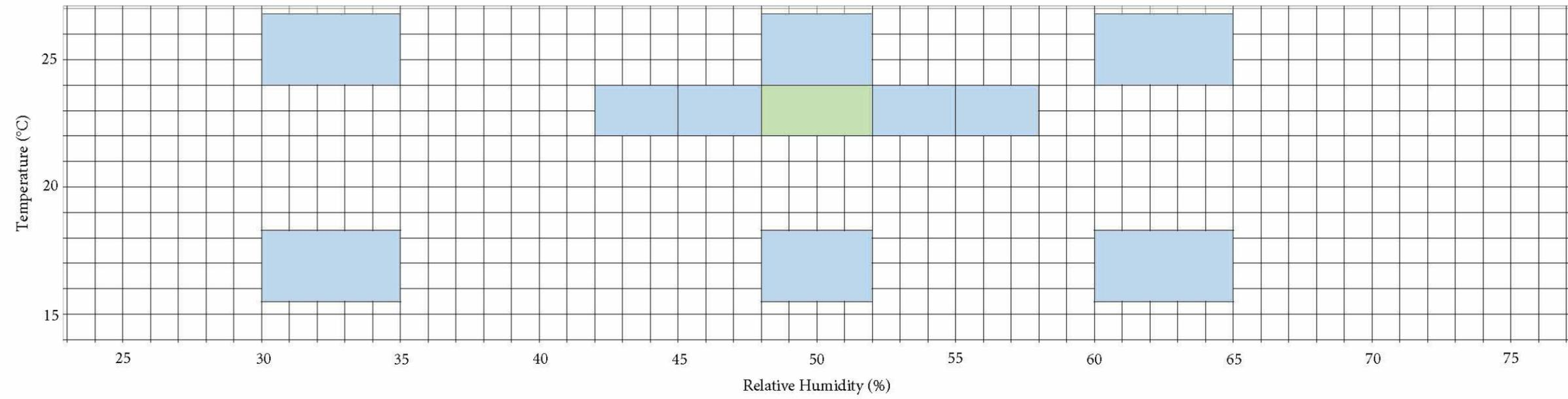
Figure A1. Target ranges for conditioning and testing environments.
