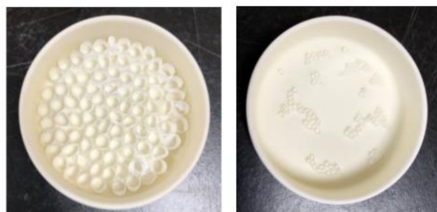
Left: Finished MTC. Right: Post heat-treated MTC
