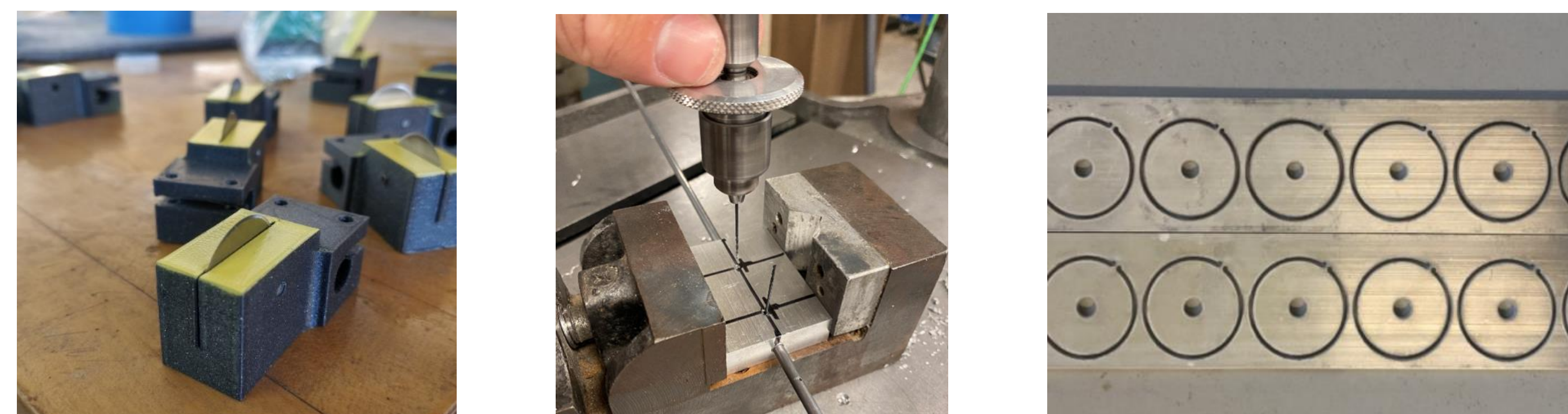
Left: Printed blade holders. Center: Mandrel manufacturing. Right: Waterjet-cut sealing disks
