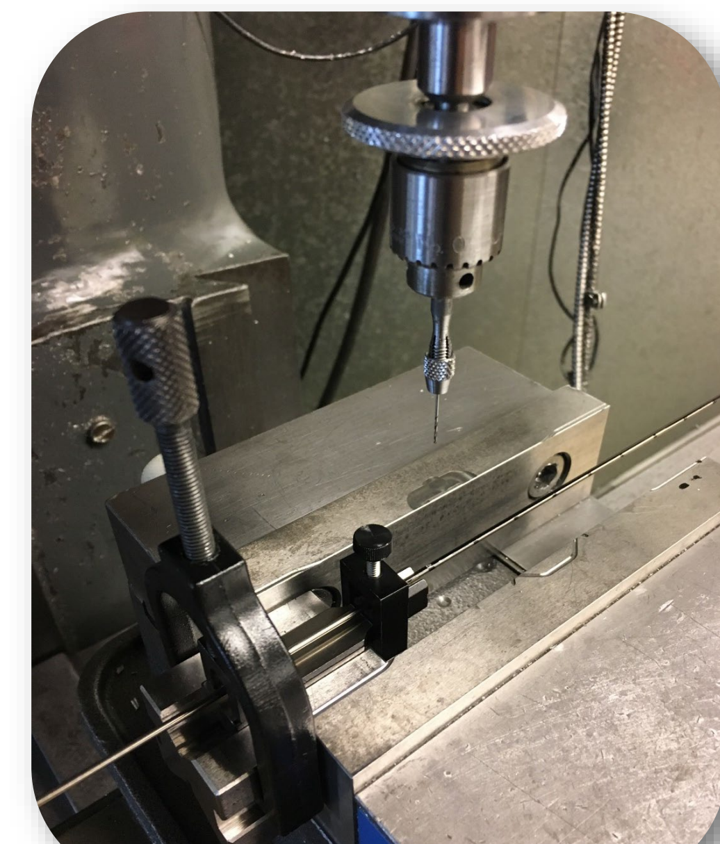
Precision Milling for Mandrel Holes
